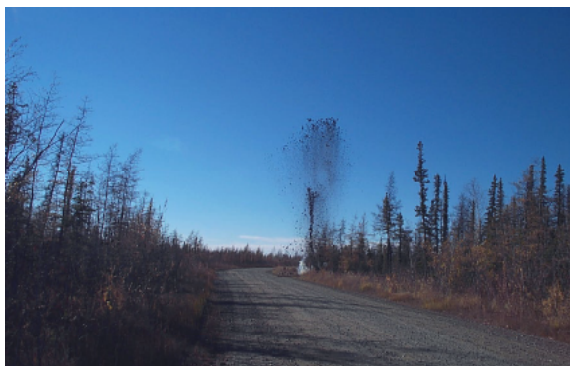
Shotpoint "blowout" during seismic acquisition
