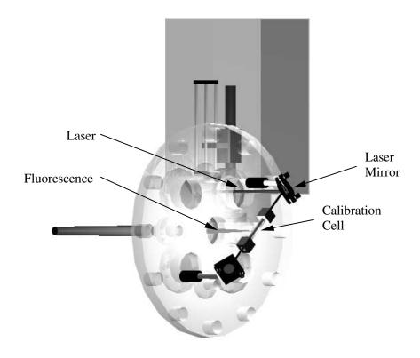
Figure 3 - Schematic of the Calibration Cell Showing Laser in Red and the Fluorescence Signal in Green.
