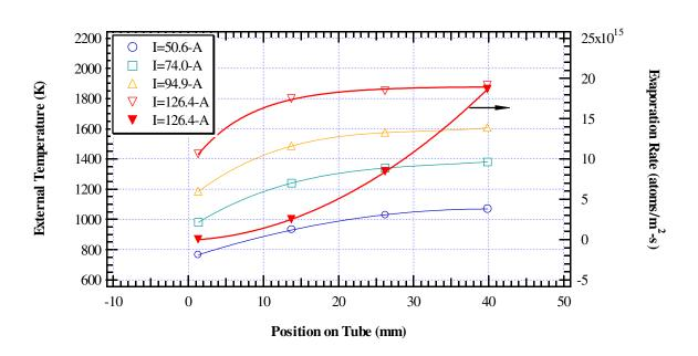
Figure 6 - Measured External Temperature Distribution for the Molybdenum Tube.
