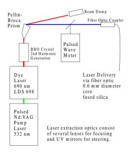
Figure 5 - Schematic of the Pulsed Laser System.
