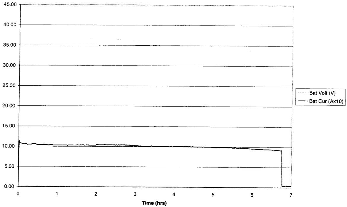
**Range Test, 0% Grade, 5 mph Initial Speed, Normal Mode**
