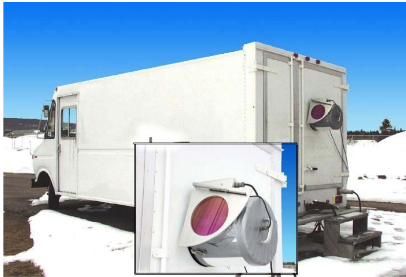
Figure 13, Canadian Defense Research Establishment, Valcartier (DREV) MFOV Lidar
