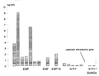
KEY: ESP=electrostatic precipitator; EGF=electrified granular bed filter; S=scrubber; FF=fabric filter; DeNOx=Thermal DeNOx.
