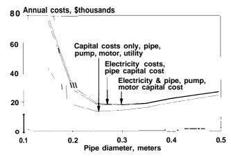
This figure shows annualized total system costs for three different types of system accounting: 1) capital rests only, including the pipe, pump, motor, and utility generation, transmission, and distribution equipment; 2) capital costs of the pipe only plus the cost of electricity; 3) capital costs of the pipe, pump, and motor plus the electricity costs to operate the system. Arrows indicate the minimum total cost for the three cases indicated.
