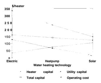
Capital costs to the individual consumer are substantially higher for solar water heaters than for electric resistance heaters. When upstream utility investment is included, however, the capital costs for solar water heaters are modestly lower than the systemwide capital costs for electric resistance and heat pump water heaters. Lifecycle operating costs to the consumer are dramatically lower for solar heaters than for electric heaters.
