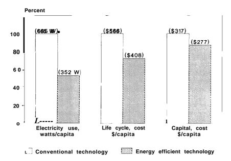
Figure 1 -I—Electricity, Life Cycle Cost, and Capital Cost Savings of High Efficiency
