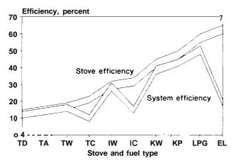
Stove efficiencies are nominal values for the stove alone; system efficiencies include the energy losses in producing, converting, and delivering fuel to the consumer. Note particularly the low system efficiencies for charcoal (TC and IC) and electric (EL) stoves due to the large energy losses in converting wood to charcoal and fuel to electricity.
