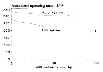
More efficient AS D/motor systems have lower annualized operating costs than less efficient motors alone.
