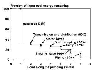
This figure shows the useful energy remaining at each stage of a pumping system. The values in parentheses are the efficiencies of the particular device at each stage.
