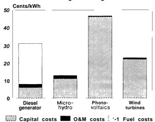
This figure compares nominal costs for different technologies where good wind, hydro, and solar resources are present. Note that these figures do not include system losses of power conditioning or battery storage and will vary widely depending on local conditions.
