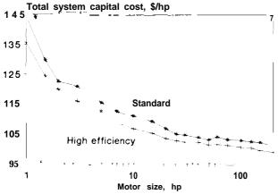
This figure shows that for all sizes of motors considered, total system capital costs are lower for high efficiency motors. Note that these values are given per horsepower of motor capacity. Large motors will cost more in total, but less per unit capacity.
