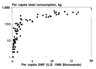
The saturation of the steel market at higher income levels as national infrastructures are developed is readily seen in linear or logarithmic plots. It is shown herein a semilog plot so as to better display both low-end and high-end data. Each data point represents a country.
