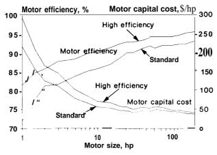
This figure shows that for all sizes of motors, high efficiency models have a higher capital cost than standard models. This additional capital cost generally decreases as motor size increases. Note that these values are given per horsepower of motor capacity. Large motors will cost more in total, but less per unit capacity.
