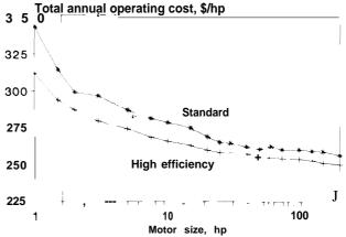
This figure shows that for all sizes of motor considered, total annual operating costs are lower for high efficiency motors. Note that these values are given per horsepower of motor capacity. SOURCE: U.S. Congress, Office of Technology Assessment, 1992. See app. A for details.
