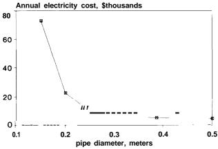
Assumptions: 6-meter static head; 30-meter friction head for 200 mm pipe diameter; 500-meter pipe; 90 l/s flow.
