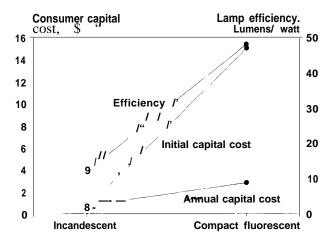
This figure indicates the barrier to buying the compact fluorescent bulb faced by the first-cost sensitive consumer. It also shows that the longer lifetime of the compact fluorescent bulb, shown on the basis of annualized capital cost, largely offsets its higher initial capital cost.
