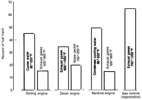
Figure 39.—Waste Heat Availability From Different Engines
