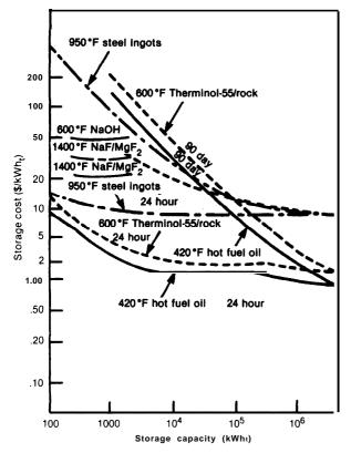
Figure 43.—High.Temperature Thermal Storage Cost per kWh.v. Storage Capacity
