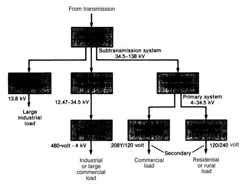
Figure 11.—Typicai Eiectric Distribution System (three.phase)
