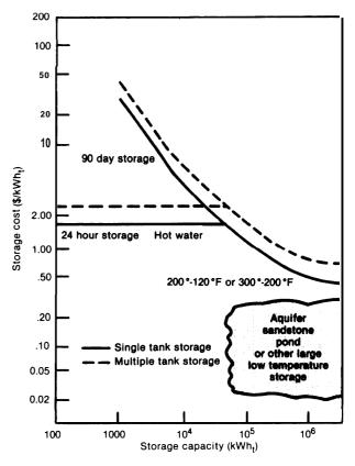
NOTE: The storage units would lose only about 5 percent of the energy stored in the interval indicated. This cost is based on precast concrete and coated steel, and excludes 25 percent O&P.
