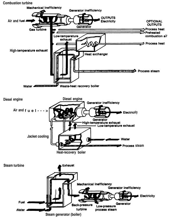
Figure 3.—illustrations of Topping Cycle Cogeneration Systems
