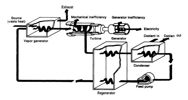
Figure 4.—Schematic of a Bottoming Cycle Cogenerator
