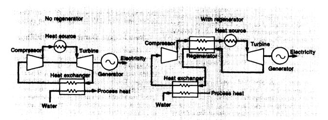
Figure 22.—Closed-Cycle Gas Turbines With and Without Regeneration
