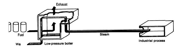
(C) Cogeneration system requires the equivalent of 2 3/4% barrels of oil to generate the same amount of energy as systems A and B
