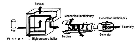
(A) Conventional electrical generating system requires the equivalent of 1 barrel of oil to Produce 800 kWh electricity
