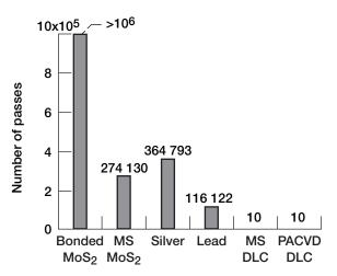
Figure 4.—Average values of endurance lives for solid lubricating films in sliding contact with 440C stainless steel balls in ultrahigh vacuum.
