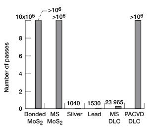
Figure 6.—Average values of endurance lives for solid lubricating films in sliding contact with 440C stainless steel balls in dry nitrogen.
