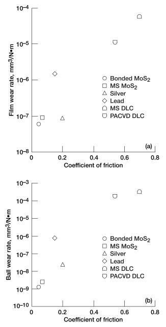
Figure 1.—Average values of steady-state (equilibrium) coefficients of friction and wear rates (dimensional wear coefficients) for solid lubricating films in sliding contact with 440C stainless steel balls in ultrahigh vacuum. (a) Film wear rate. (b) Ball wear rate.
