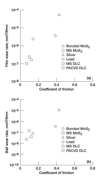
Figure 2.—Average values of steady-state (equilibrium) coefficients of friction and wear rates (dimensional wear coefficients) for solid lubricating films in sliding contact with 440C stainless steel balls in humid air. (a) Film wear rate. (b) Ball wear rate.
