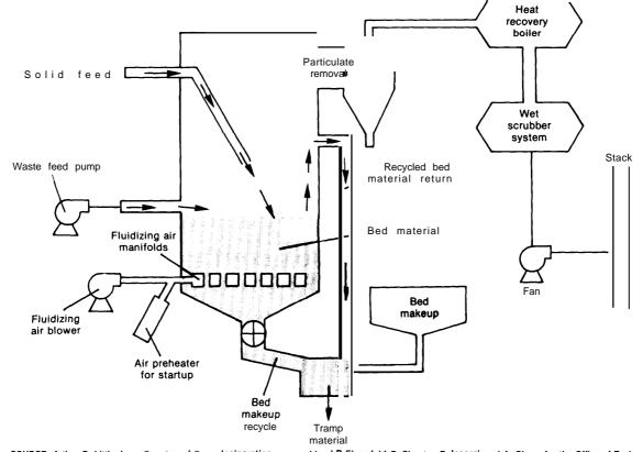
Figure 5.— Fluidized Bed Incineration Technology
