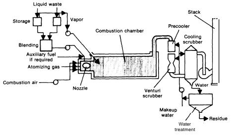
Figure 3.—Liquid Injection Incineration Technology
