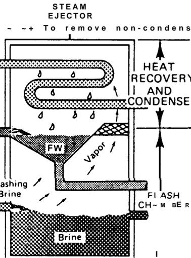
Tube bundle which serves as a heat recovery and condenser section. Incoming seawater inside the tubes is heated by vapor condensing on the outside of the tubes.
