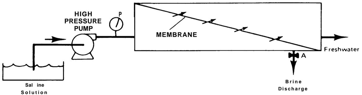
A membrane assembly is generally symbolized as a rectangular box with a diagonal line across it representing the membrane.
