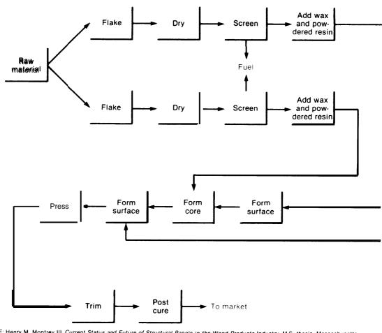
Figure 17.— Idealized Typical Waferboard Process
