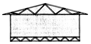
This truss framed system combines floor, walls, and roof into a unitized framp for Struct Ura I cent in uity from the foun dation u Dtothe ridGe
