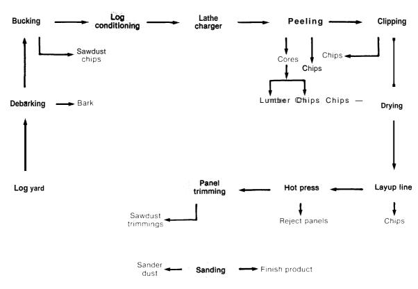
Figure 13.— Flow Diagram of a Small-Log Plywood Mill
