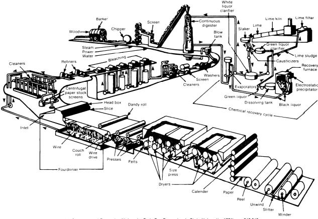
Figure 26.—Overall View of Papermaking From Chemical Pulp by the Kraft Pulping Process
