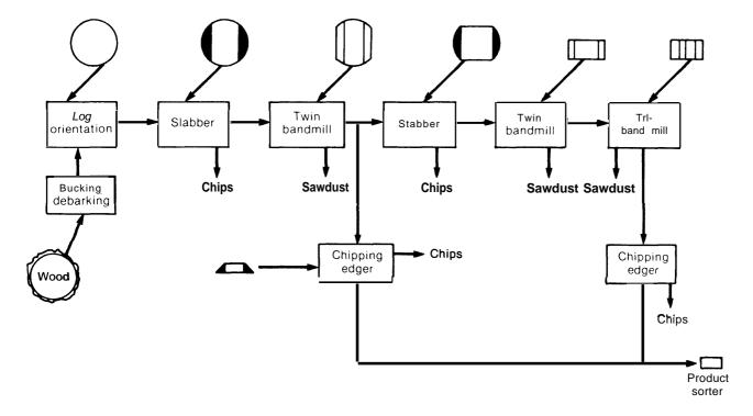
NOTE" A log profile is shown aBach machine (top) The shaded areas Indicate material which is chipped away, whenticlelines in other cross-sections indicate saw lines SOURCE" E M Williston, Lumber Manufacturing: The Design and Operation of Sawmills and Paper Mills (San Francisco. Miller Freeman Publications, 1976).
