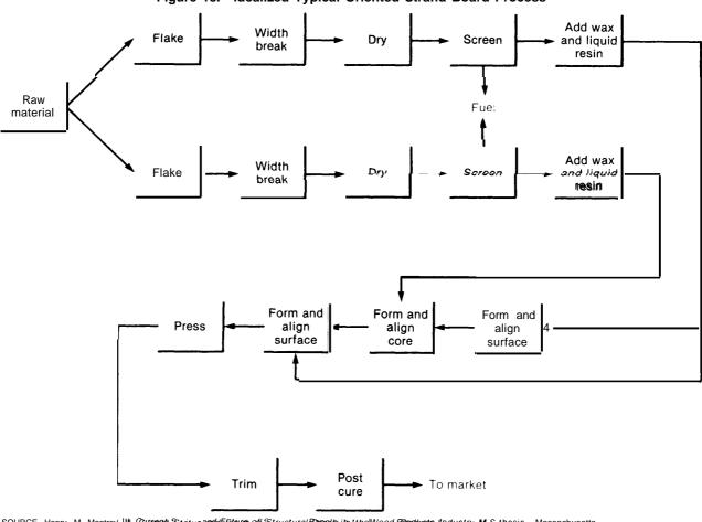
Figure 18.—Idealized Typical Oriented Strand Board Process
