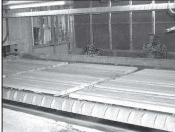
Figure 11.—Case-finishing (left) versus component flat-line finishing (right).
