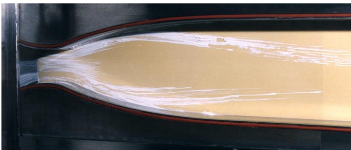
Fig. 4 Sidewall boundary layer flow pattern.
