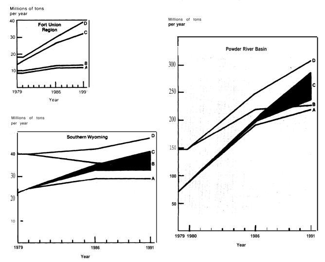
Figure I0.—Planned Capacity and Potential Production of All Mines With Federal Leases in the Powder River Basin, Southern Wyoming, and Fort Union Region
