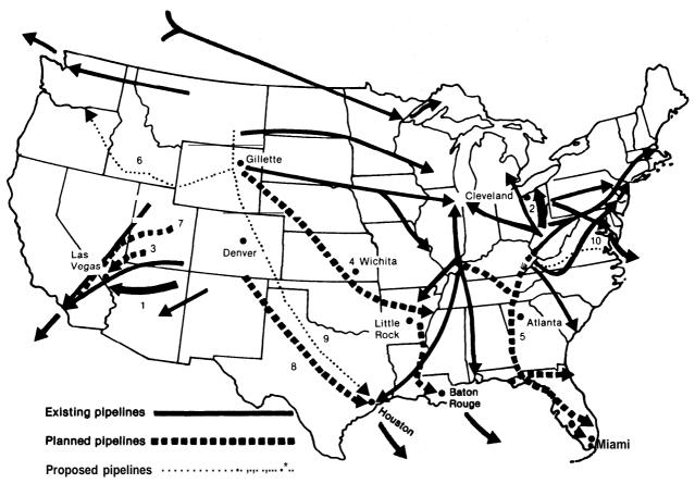
Figure 39.—Coal Slurry Pipeline Systems
