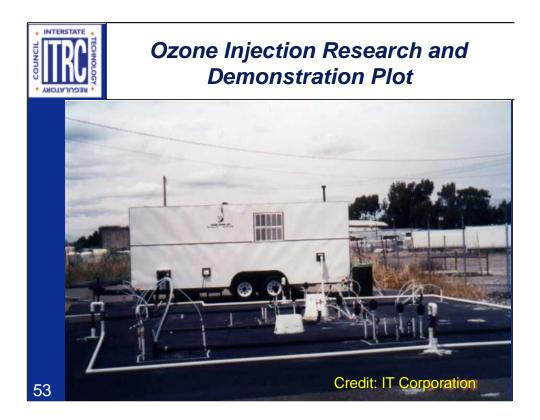
Manifold system and injection points are visible in the foreground.
