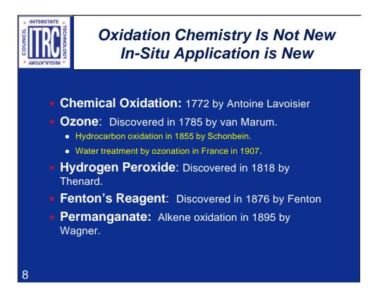
As you can see, the concept of chemical oxidation is not new, and in fact has been established for >225 years. The new part is the application of oxidant chemicals to contaminants in situ.
