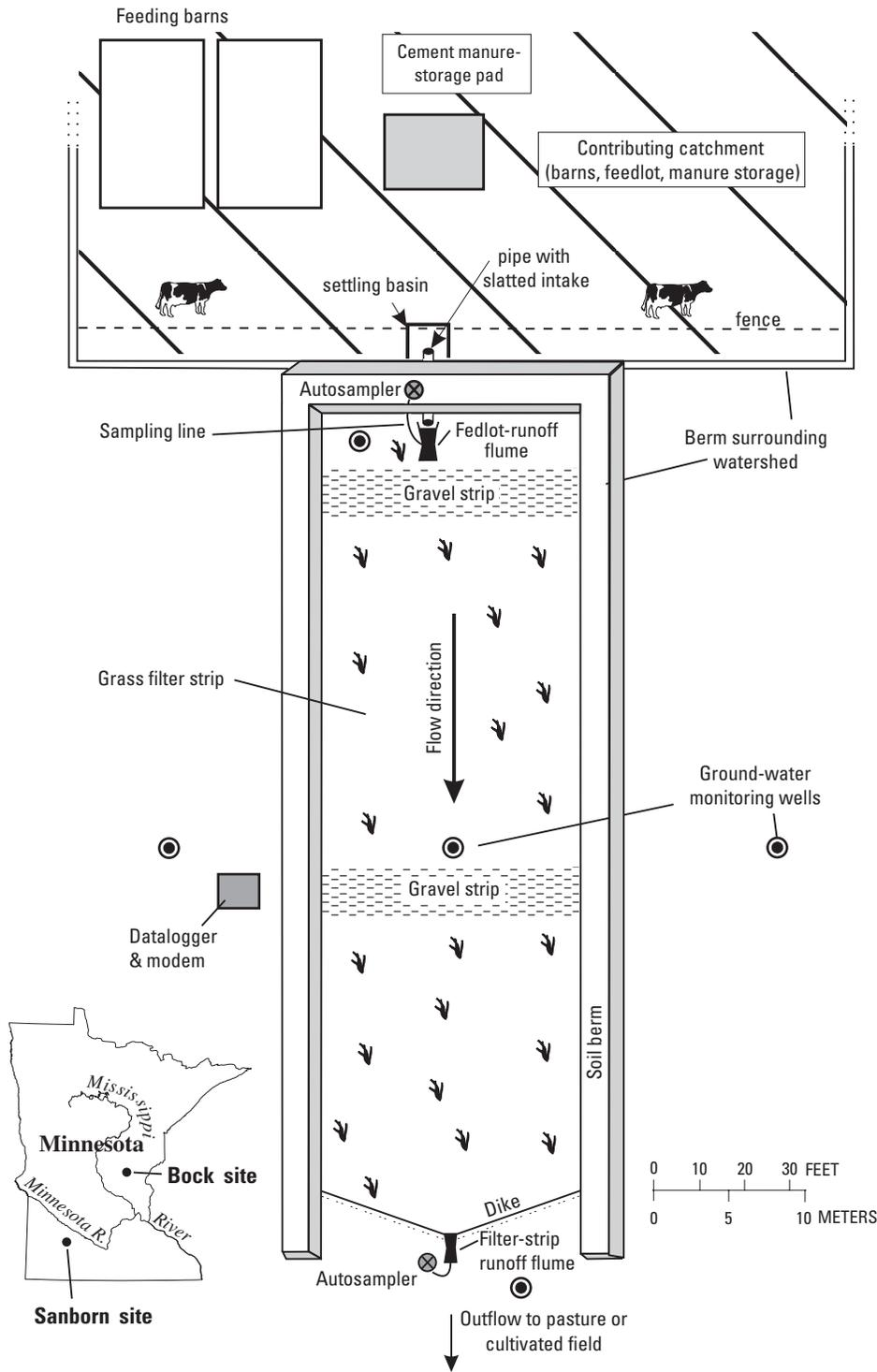
**Figure 1.** Plan view of filter strips at Bock and Sanborn, Minnesota sites.
