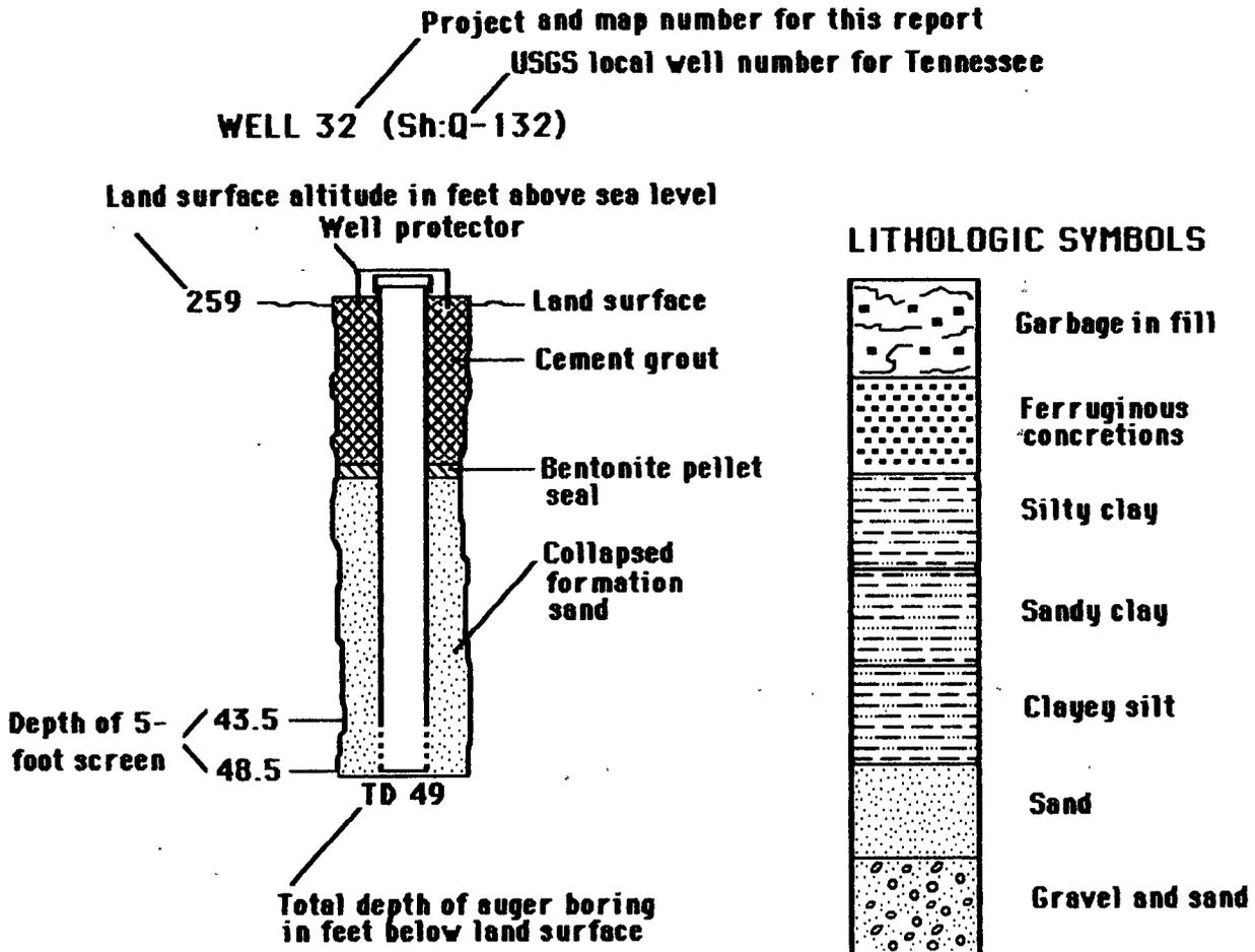
Observation wells in the alluvial aquifer are constructed with 2-inch-diameter, polyvinyl chloride (PVC) casings and screens. Most wells were developed by evacuating at least five volumes of water with a low-capacity (about 1 gallon per minute) submersible pump.
