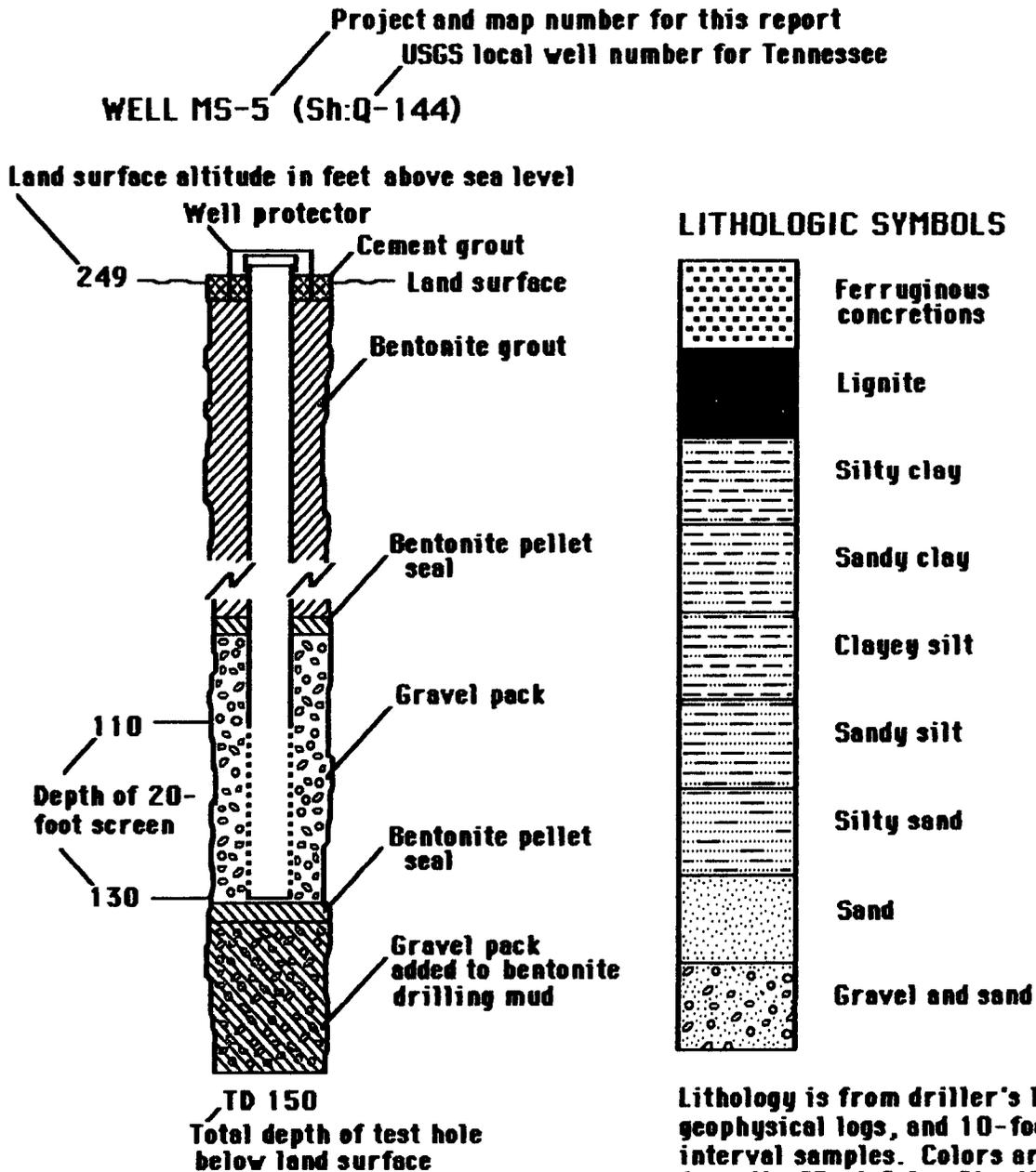
Observation wells in the Memphis aquifer are constructed with 4-inch-diameter, polyvinyl chloride (PVC) casings and screens. Wells were developed at least 1 hour by pumping with air compressor.
