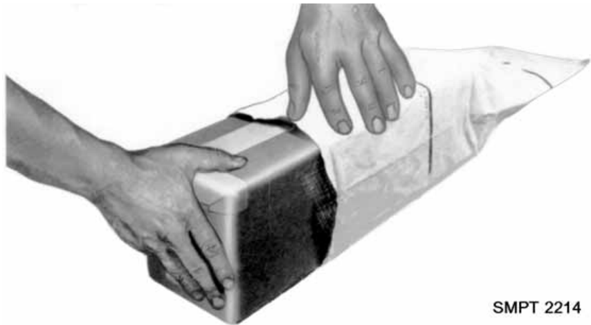
Figure 2-45. Watervaporproof bag (MIL-PRF-131, Class 1).
