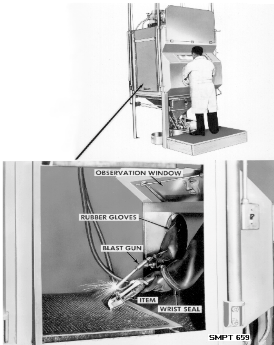
Figure 2-26. Abrasive blast cleaning honing process.
