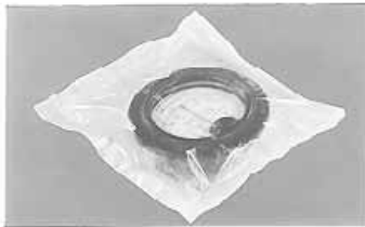
TYPE I WATER VAPORPROOF, WATERPROOF, GREASEPROOF THIS BARRIER MATERIAL IS USED FOR METHOD 41 AND METHOD 51.
