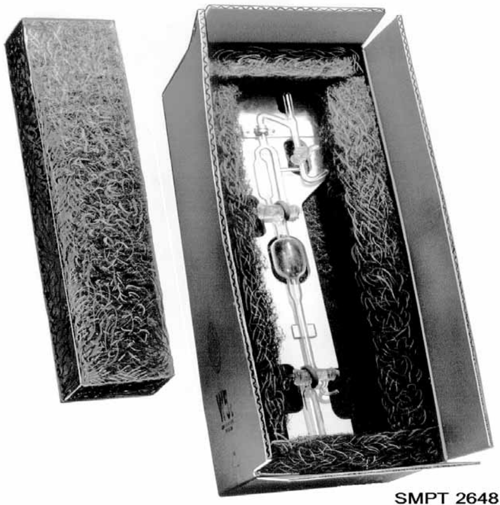
Figure 2-54. Cushioning used to control movement.
