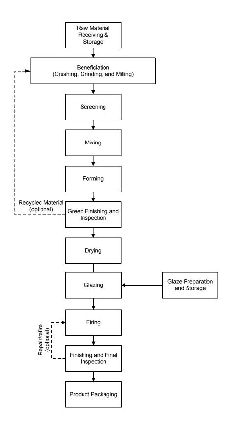
Figure 2-1. Ceramics Process Flow Diagram
