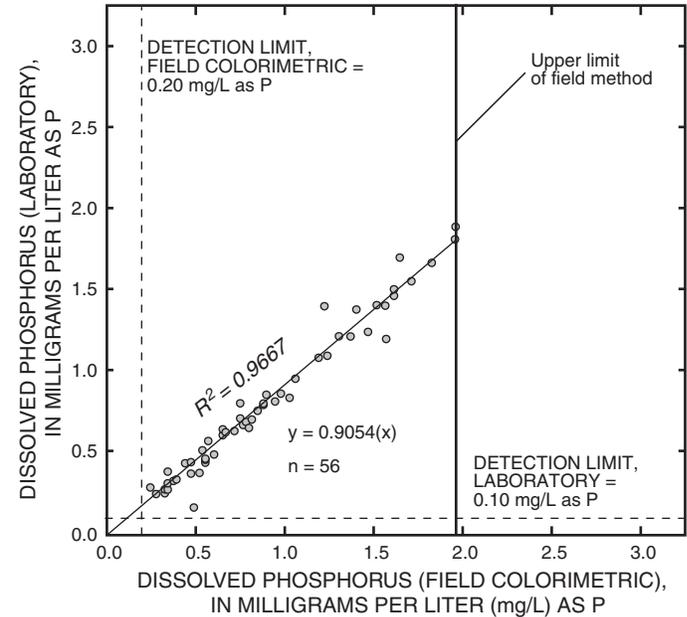
**Figure 6.** Comparison of field- and laboratory-determined dissolved phosphorus concentrations in pond-bottom ground water in the contaminant-plume discharge area, Ashumet Pond, Massachusetts, 1999.
