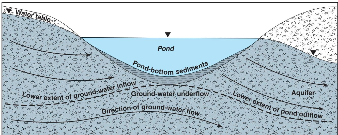
**Figure 4.** Conceptual model of the ground-water-flow system near a glacial-kettle ground-water flow-through pond.
