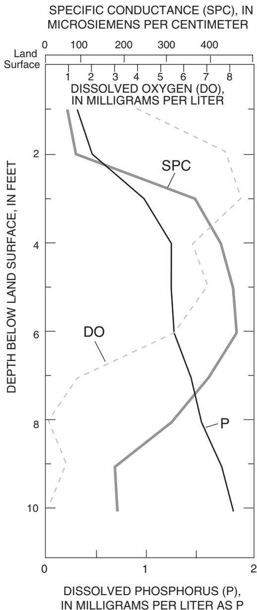
**Figure 11.** Distribution of dissolved phosphorus, specific conductance, and dissolved oxygen at a vertical profile (3a-00-ST) at the shoreline of Ashumet Pond, Massachusetts, August 24, 1999 (location of profile shown in fig. 5).
