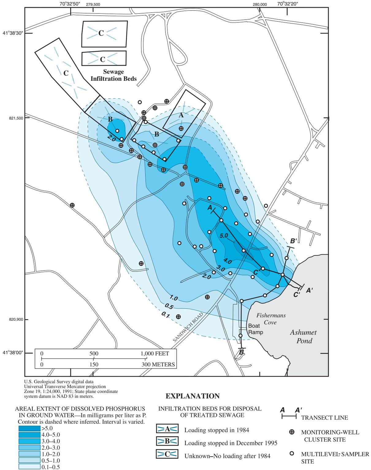
**Figure 7.** Areal distribution of maximum dissolved phosphorus concentrations in ground water upgradient of Ashumet Pond, Massachusetts, April–July 1999.
