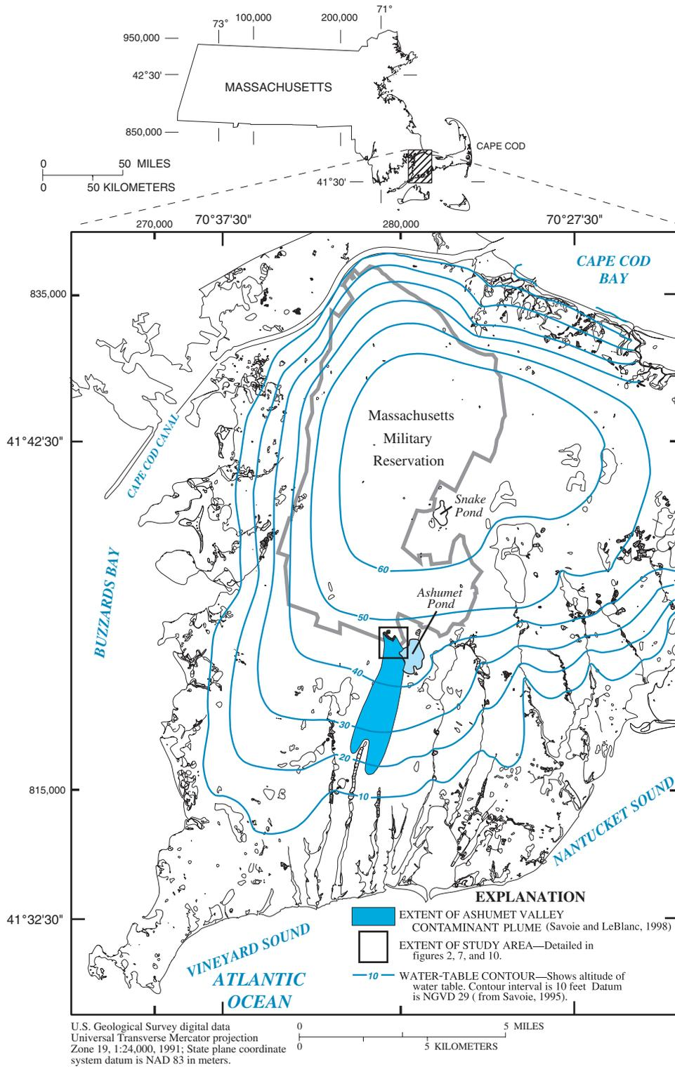
**Figure 1.** Location of the Massachusetts Military Reservation, extent of the contaminant plume, and the altitude of the water table, western Cape Cod, Massachusetts.
