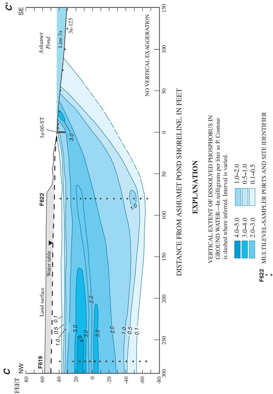
**Figure 12.** Vertical distribution of dissolved phosphorus concentrations along section C-C' from multilevel sampler F619 to pond-bottom location 3a-125, Ashumet Pond, Massachusetts, April–October 1999 (location of profile shown in fig. 7).
