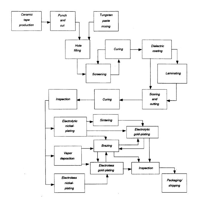
Figure 1. Abbreviated Process Flow Diagram for production of mountings for electronic circuit components.
