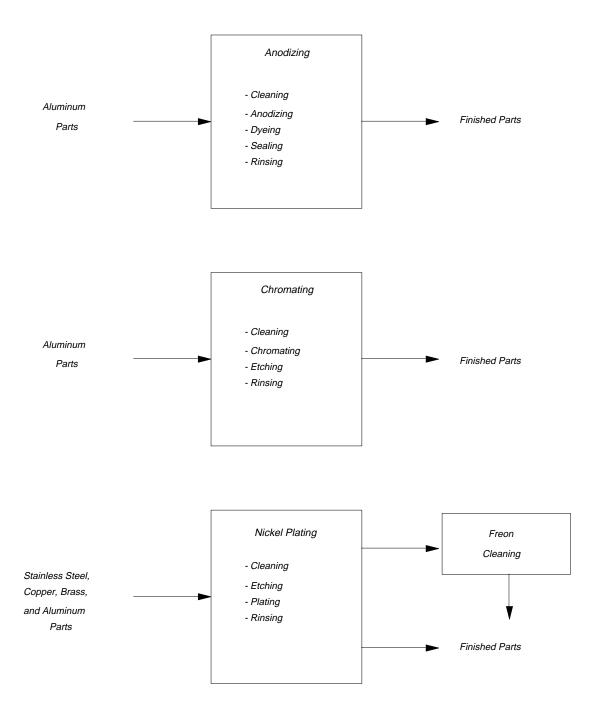
Figure 1. Abbreviated process flow diagram for metal parts coating.
