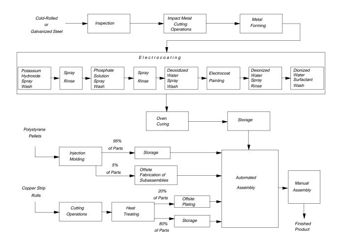
Figure 1. Abbreviated process flow diagram for electrical load center manufacture.
