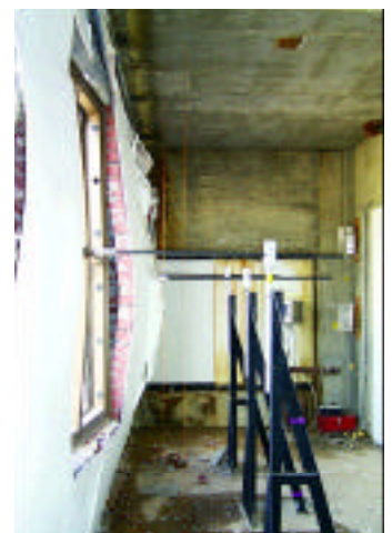
Figure 10. Post-test Photos of the of the Sheet Steel Wall Retrofit.
