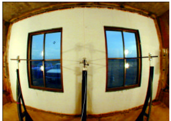
Figure 9. Pre-test Photos of the Sheet Steel Wall Retrofit.
