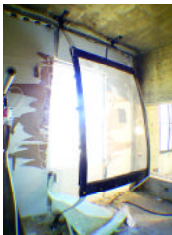
Figure 7. Pre- and Post-test Photos of Interior View of 3/4" Polycarbonate Window, Secured Using Steel Straps, Anchored at Floor and Ceiling Using 3" x 1/4" Steel Straps.
