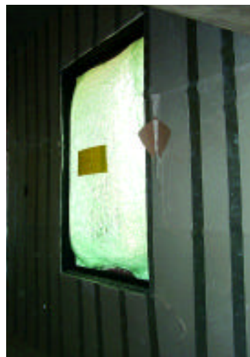
Figure 13. Post-test Photos of Steel Stud Retrofit Wall with Windows.
