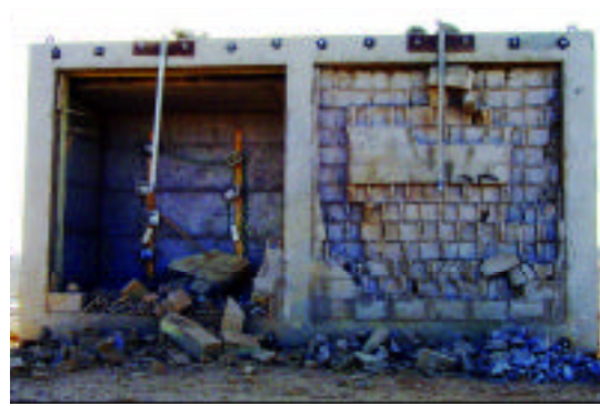
Figure 14. Pre- and Post-test Photos of Cubicle Three, the Right Half of Which Was Retrofitted with Spray-on Elasto-polymer.
