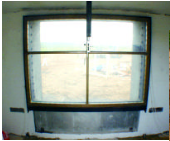
Figure 8. Pre- and Post-test Photos of the Structural Muntin Frame System Installed as a Retrofit.
