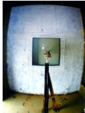
Figure 16. Pre- and Post-test Photos of the Interior of a Reinforced Concrete Wall Containing a Window Retrofit Using Spray-on Elasto-polymer to Catch the Window During Blast Loading.
