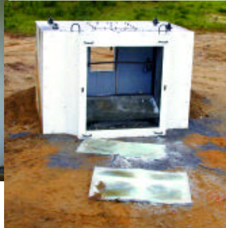
Figure 8. Pre- and Post-test Photos of the Structural Muntin Frame System Installed as a Retrofit.
