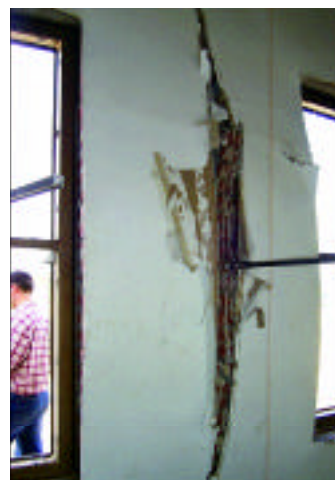
Figure 10. Post-test Photos of the of the Sheet Steel Wall Retrofit.
