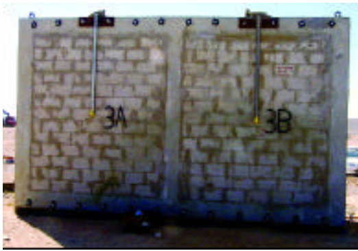
Figure 14. Pre- and Post-test Photos of Cubicle Three, the Right Half of Which Was Retrofitted with Spray-on Elasto-polymer.
