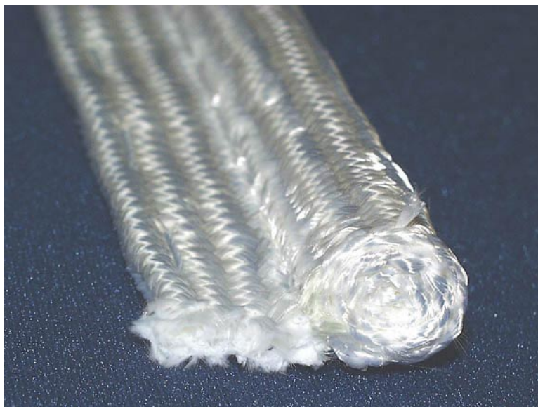
Figure 18.—End View of a Typical Seal Assembly After Sizing Removal, But Prior to Rigidization of the “Tail.”
