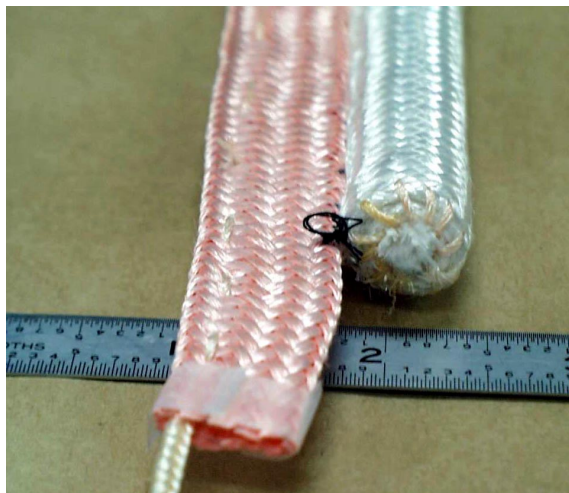
Figure 15.—End View of Seal Assembly Showing End Closure and Attachment “Tail” Prior to Sizing Burnout.
