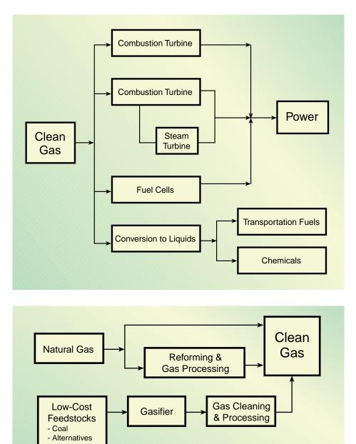
Clean gas is used as a feedstock for coproduction, including power generation and conversion to transportation fuels and chemicals.
