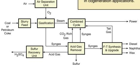
Texaco Energy Systems process flow diagram
