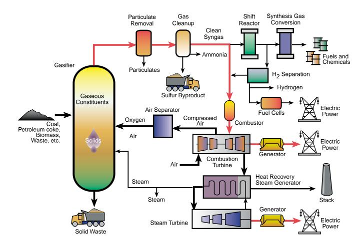
other gases such as carbon dioxide  $(CO_2)$ , hydrogen sulfide  $(H_2S)$ , ammonia  $(NH_3)$ , water vapor, and methane  $(CH_4)$ , with traces of other materials. This gas is cleaned of its contaminants and used for electric power production. Such a system is inherently more efficient and cleaner than conventional PCfired systems, with efficiencies typically being above 40% and emissions reduced to the lowest levels currently achievable.
