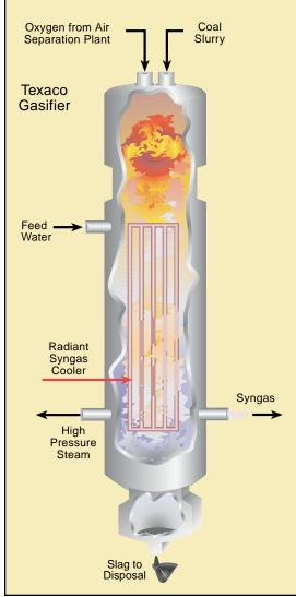
ers to produce a fuel for gas turbinebased electric power generation; the gas turbine exhaust produces steam to generate additional electricity.
