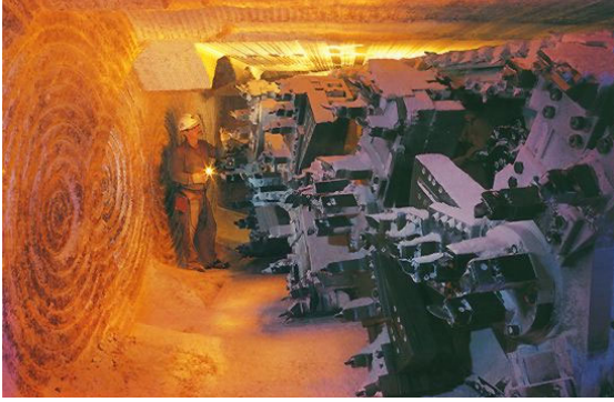
Figure 11. Continuous miner at Rocanville potash mine, Saskatchewan. (Net Resources International Limited)
