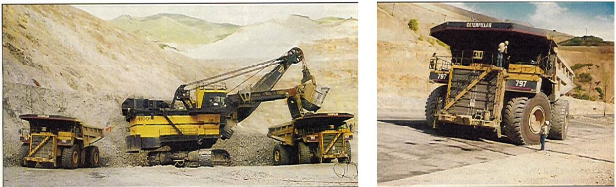
Figure 10. Shovel loading 360-ton trucks at Bingham Canyon copper mine, Utah. (Rocky Mountain Construction, August 14, 2000, p. 9.)
