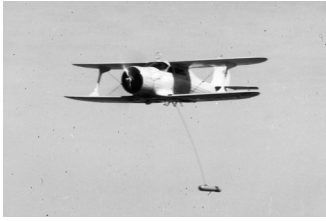
Figure 19. Beach Staggerwing aircraft conducting early geophysical survey, circa 1949. (Photo courtesy of V. Labson, USGS.)
