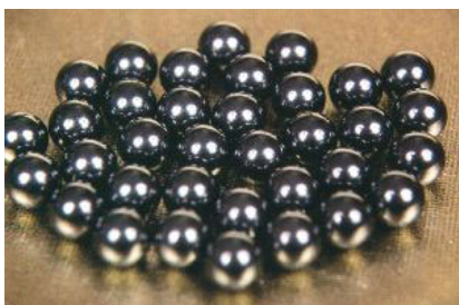
Figure 14. Diamond coatings on ball bearings improve wear characteristics. (Photo from Refmet Ceramics Limited, Advanced Surface Technologies: Refmet Ceramics Limited web site at http://www.diamond-like-carbon.com/wear.htm . (Accessed March 23, 2001.)
