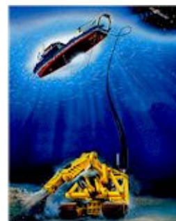
Figure 13. Diamonds are recovered from waters off the coast of Namibia by a remote controlled vehicle traveling along the ocean bed. (Photo from JDR Cable Systems, Communication Lines: JDE Cable Systems web site at http://www.jdr cables.com/news/online9.asp . (Accessed September 11, 2000.)
