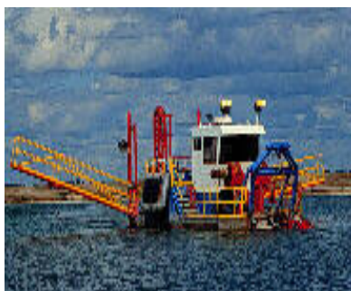
Figure 50, A floating dredge recovers potash crystals from the bottom of a 130 acre cooling pond at the Belle Plaine solution mine in Canada. (Photo courtesy of IMC Global Inc., 2000, Production techniques: IMC Global web site at http://www.imcglobal.com/potash/production/techniques.html . (Accessed August 24, 2000.)
