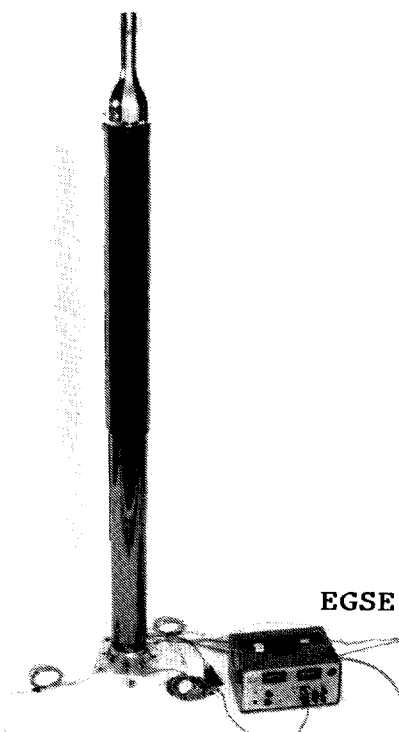
Figure 3. - S-Band antenna boom in deployed condition.
