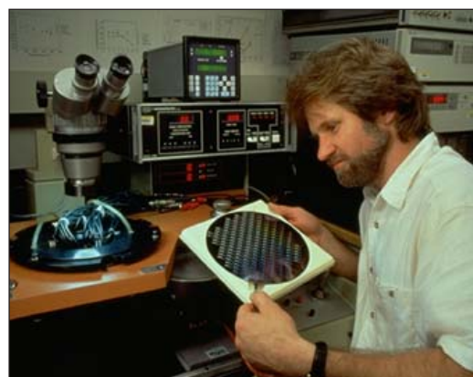
Test wafer being loaded on wafer probe for long-term dielectric testing.
