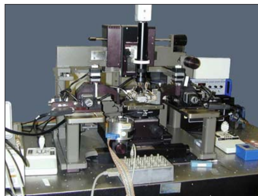
Figure 1. Universal test bed for electric and magnetic field probing on a nanoscale.
