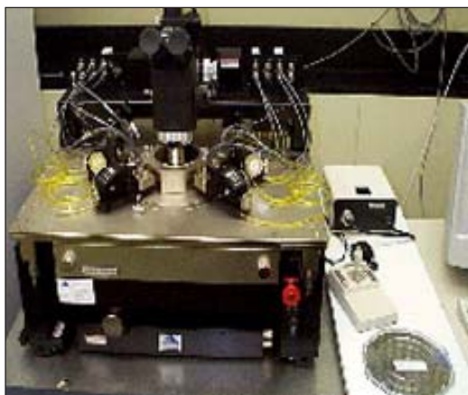
Figure 8. A low-noise ( fA ), high temperature (300 °C) probe station is used for electrical characterization of devices.
