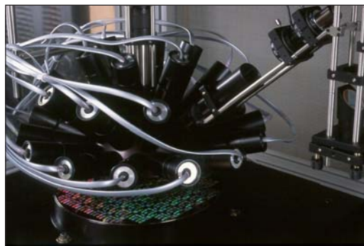
Figure 2. The MHPOSI enables the scattering from individual particles to be analyzed.
