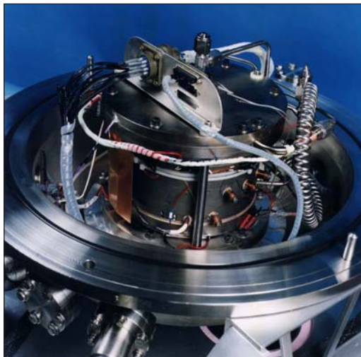
Figure 1. NIST Low Frost-Point Humidity Generator.
