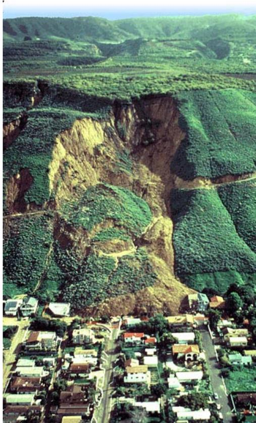
After excessive rainfall in the spring of 1995, the hillside above La Conchita, California, gave way; 600,000 tons of mud and silt partially buried the neighborhood.
