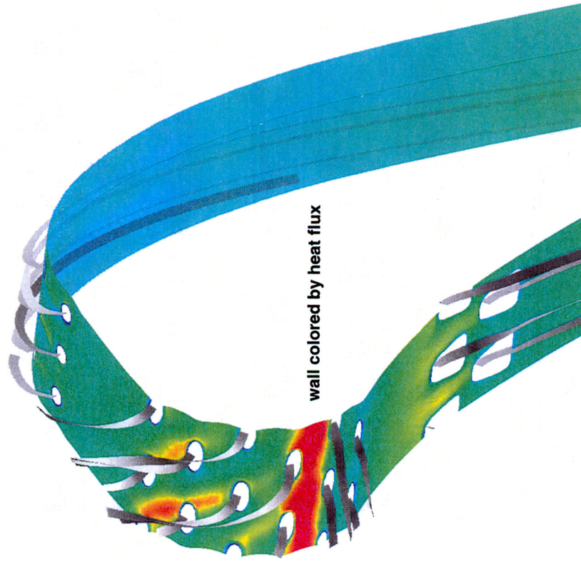
Fig. 24 Coolant streamlines out of hole-exits (Heidmann et al., 2000)
