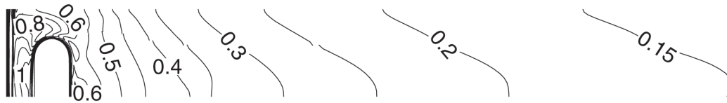
Fig. 15(b) Cooling effectiveness distribution over the surface (Ameri & Rigby, 1999)
