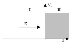
Figure 2. Particle incident on a potential step.
