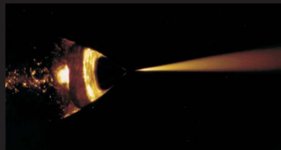
A microneutron thruster test firing, a technology required for the LISA mission.
