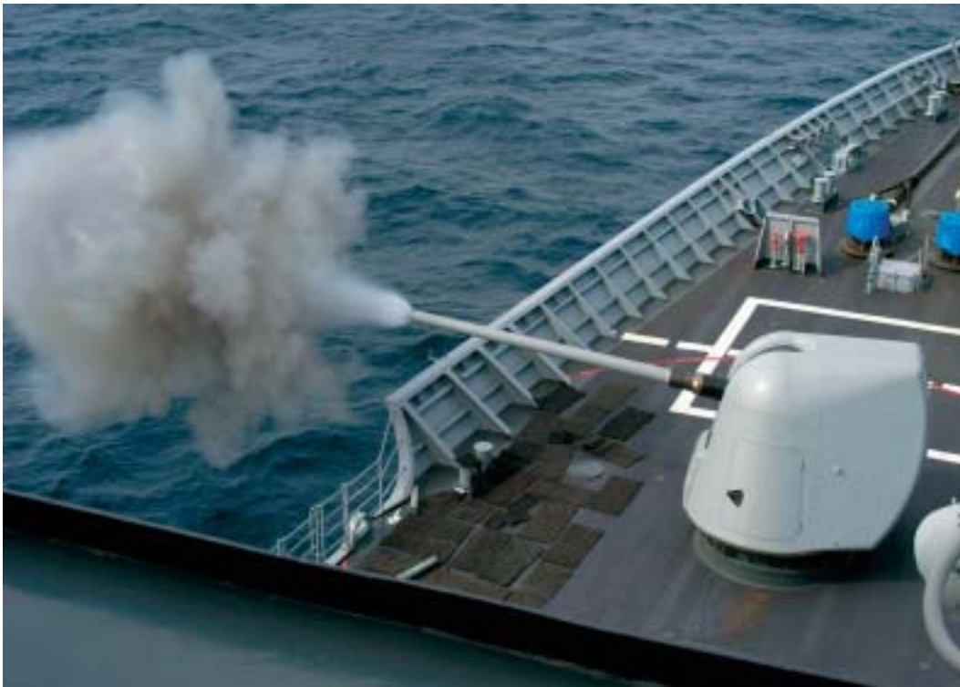
The 54-caliber (Mk 45) lightweight gun provides surface combatants accurate naval gunfire against fast, highly maneuverable surface targets, air threats and shore targets during amphibious operations.
