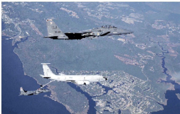
A KC-135 boom type aircraft refueling an F-15E.
