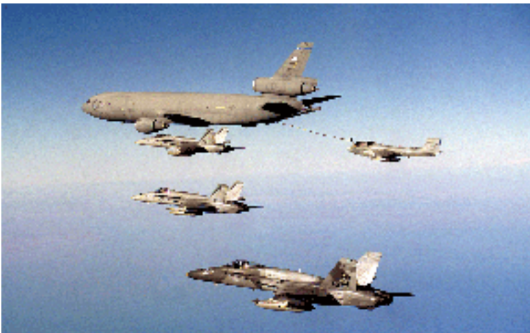
A KC-10 conducts drogue refueling operations.
