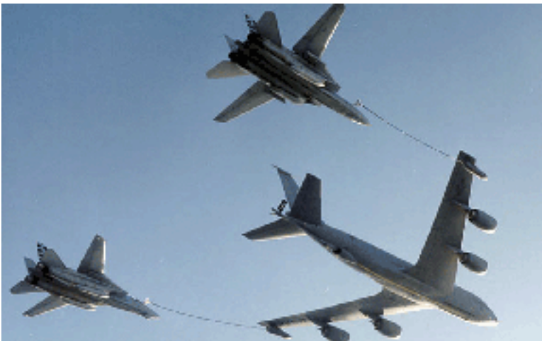
US Navy receiver aircraft using drogue air refueling procedures.
