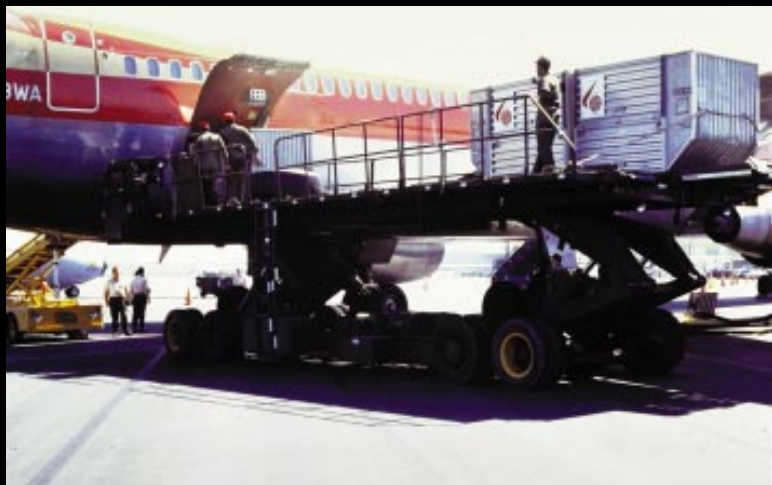
Figure II-40. 40,000-Pound 463L Aircraft Loader
