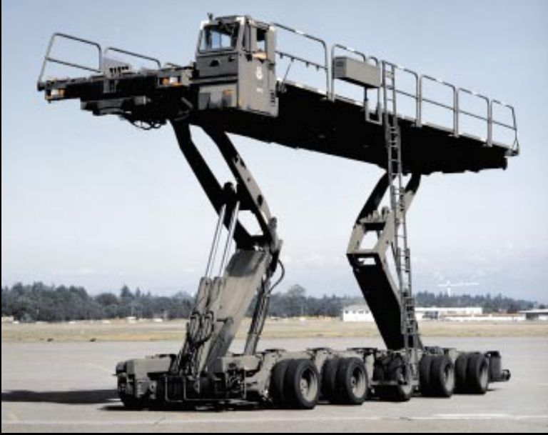
Figure II-38. 60,000-Pound 463L Aircraft Loader
