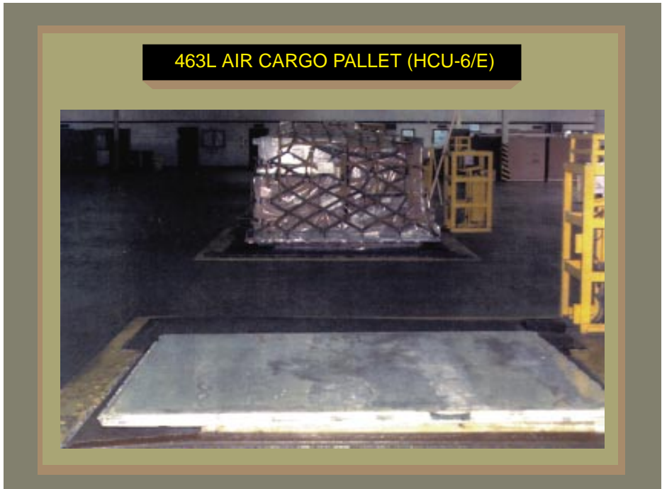
Figure II-37. 463L Air Cargo Pallet (HCU-6/E)
