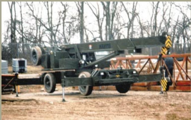
Figure II-21. 14-Ton Wheel Mounted Container Handling Crane
