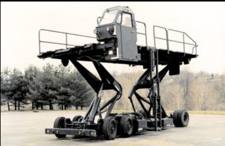
Figure II-39. 25,000-Pound 463L Aircraft Loader
