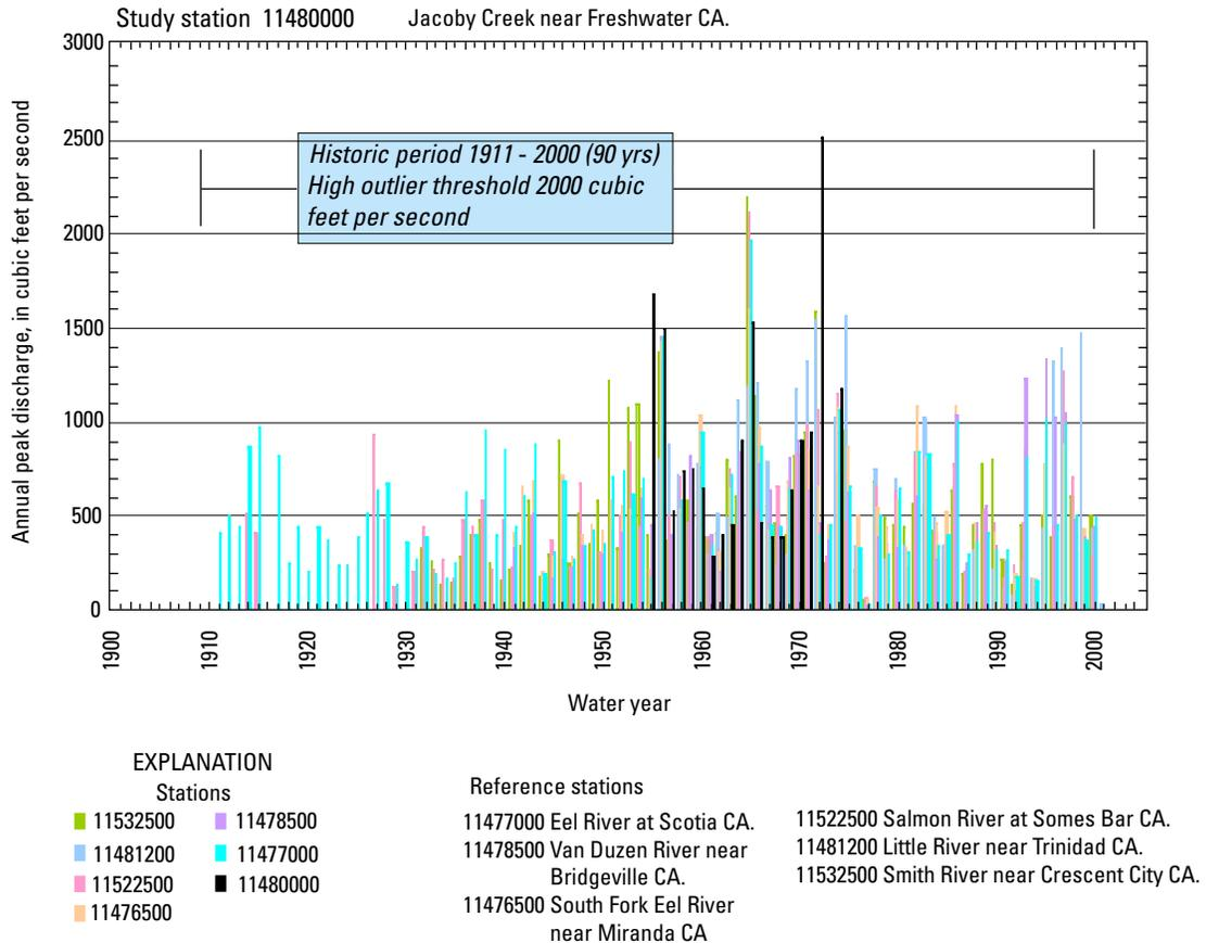
Figure 9. Graphical determination of high-outlier threshold and historic period for flood-frequency analysis.
