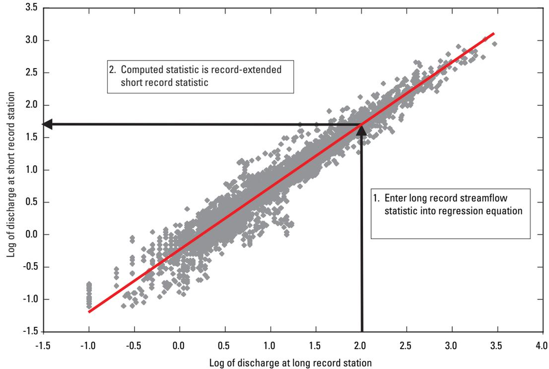
**Figure 7.** Example of extension of streamflow statistics for a short record station, using streamflow statistics from a long-record station.
