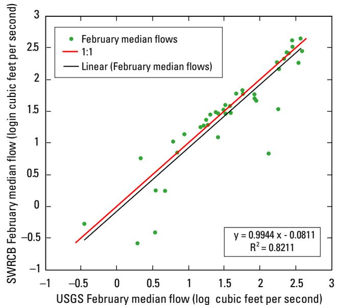
Figure 16. SWRCB flow-based February median flow estimates versus USGS February median flows for all 40 study stations.
