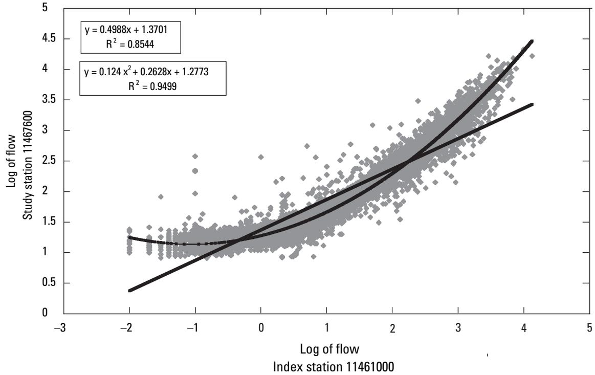
Figure 5. Example of curved versus straight-line relationship of study-station flow and index-station flow.
