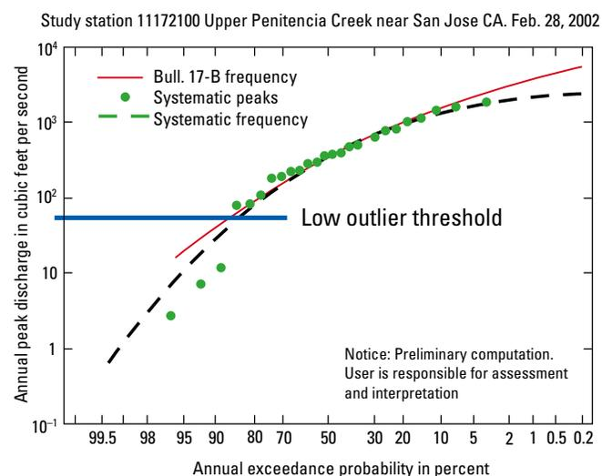
**Figure 8.** Example of graphical determination of low-outlier threshold for flood-frequency analysis.
