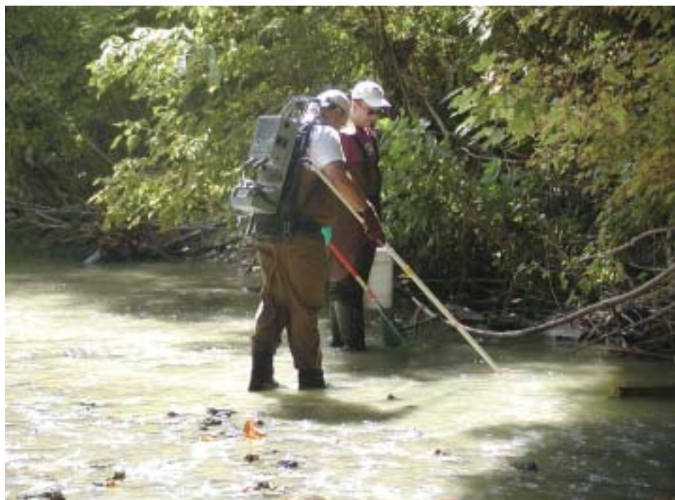
Figure 3-5. Backpack electroshocking for central stonerollers.
