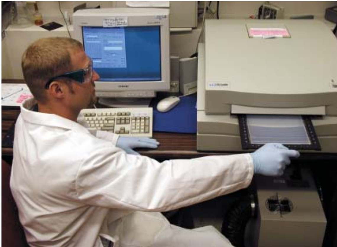
Figure 4-7. DNA quantitation is performed using a commercially available fluorescent nucleic acid stain that is detected with a fluorescent scanner.
