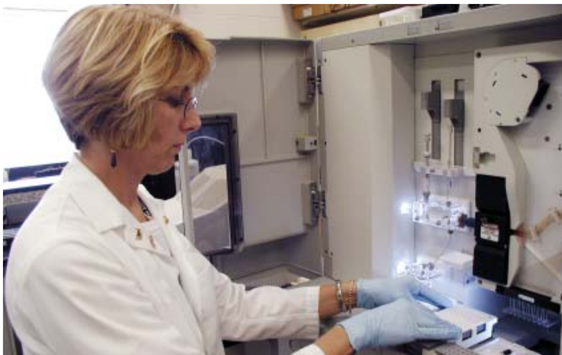
Figure 4-9. A capillary-based, auto-loading genetic analyzer can perform both fragment analysis (AFLP, microsatellite) and DNA sequencing.
