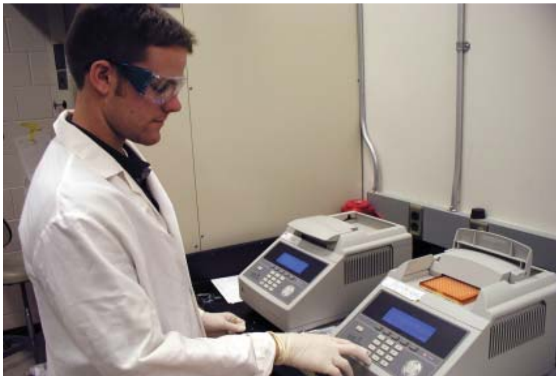
Figure 4-8. Thermal cyclers are used for fragment amplification (RAPD, AFLP, microsatellites) and DNA sequencing assays.
