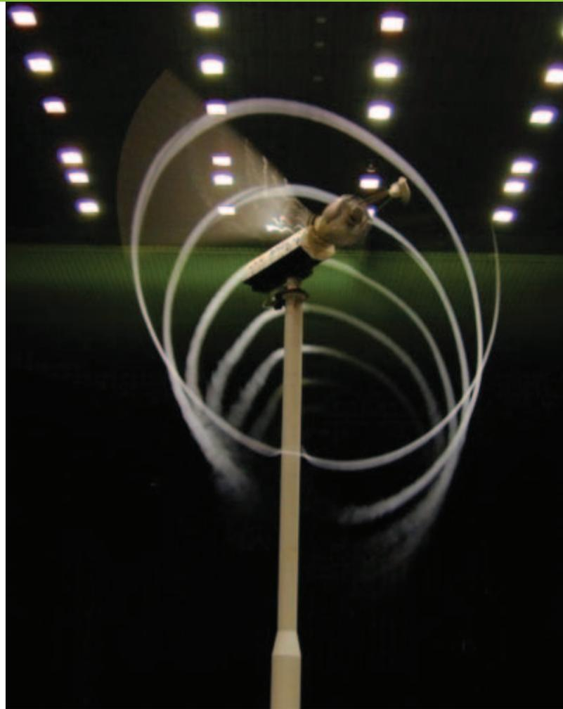
To understand wind turbine aerodynamics, researchers at NREL and SNL are combining two-dimensional field and wind tunnel test data to predict aerodynamic loads on turbines under varied inflow conditions.
