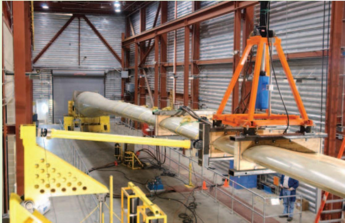
The new system, which can test blades as long as 70 m (230 ft), is the only one of its kind in the world. In December 2003, NREL researchers completed a fatigue test using the new system on a 37-m (121.4-ft) blade built by GE Wind. The completion of this first test validated the operation of the new system, and in 2004, they will begin running fatigue tests on 34- and 45-m (111.5- and 147.6-ft) blades.
