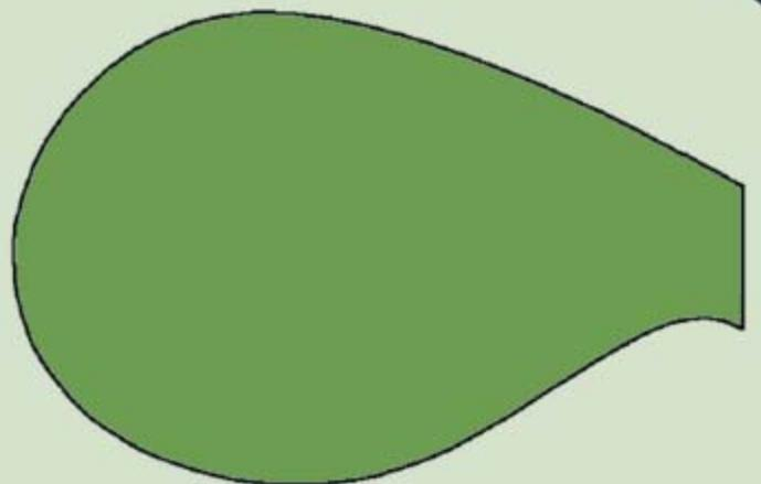
In 2004, Sandia plans to pursue innovative blade shapes that incorporate blunt trailing edges to improve the structure, simplify the manufacturing, and reduce the weight without sacrificing the aerodynamic performance.
