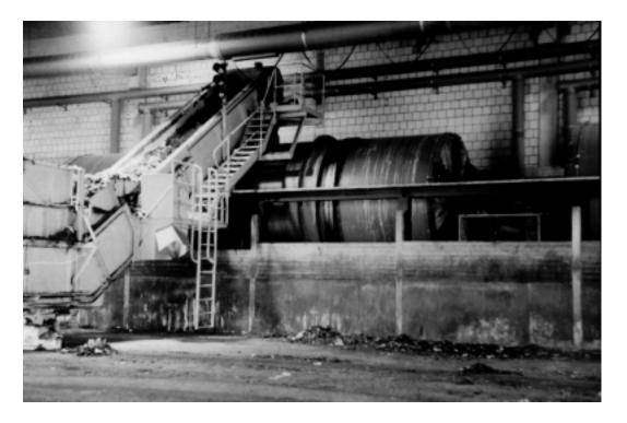
The drum temperature and oxygen content are monitored continuously, and air addition and mixing are done as needed to maintain conditions within designated ranges.
