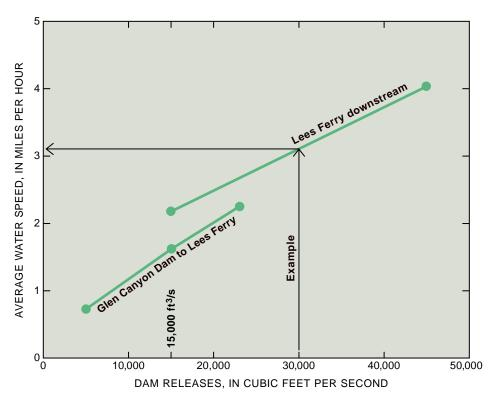
Water speed from the dam to Lees Ferry has been measured at three dam releases and downstream from Lees Ferry at two releases. Water moves a little more slowly upstream from Lees Ferry than downstream. We can use the results to estimate the average water speed for a range of constant discharges. For example, the data indicate that at 30,000 ft <sup>3</sup>/s water would flow downstream from Lees Ferry at a little more than 3 mph.
