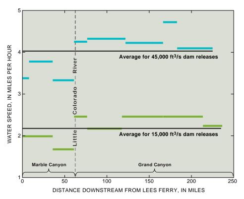
Water speed through reaches defined by sampling sites was less than the average for Marble Canyon and equal to or greater than the average for Grand Ca nyon for both constant dam releases measured.
