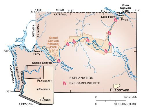
Dye movement was tracked by sampling the water and measuring the dye concentration at eight sites during the controlled flood.
