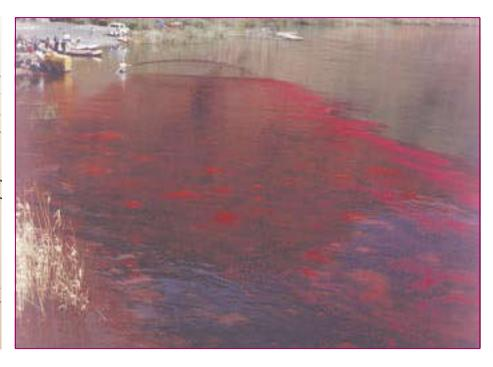
Athough the dye is easy to see where it is first put into the river, it quickly mixes with the much larger mass of river water and becomes invisible. The highest concentration at sampling sites was between 5 and 35 parts per billion. One part per billion is about equal to one drop in a backyard swimming pool.
