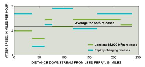
Water speed measured in reaches between sampling sites was either higher or lower at rapidly changing releases than at constant releases, depending on whether the dyed water moved through the reach with the peak or trough of the discharge wave.
