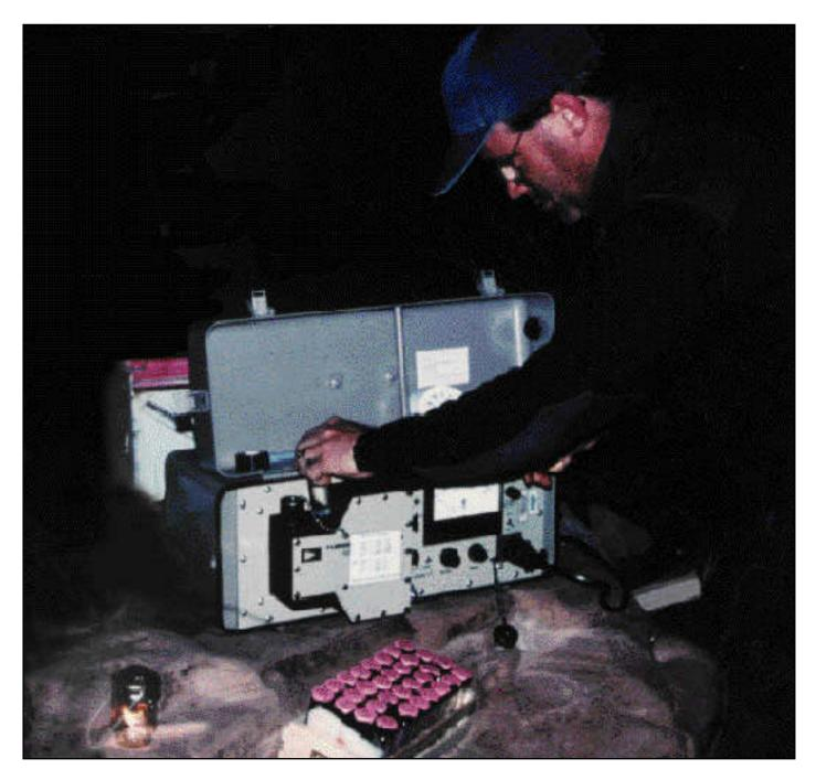
At each site, water samples were collected from near the riverbank during passage of the dye and measured in the field for dye concentration using a fluorometer. At the site pictured, the dye concentration peaked at around midnight. Samples from all sites were retained and remeasured in the lab under controlled tem perature conditions to obtain the final concentrations.
