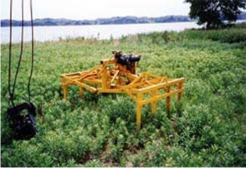
Figure 4. Commercially manufactured hay bale tongs for a crane. Were these actually attached to a crane, they would be hydraulically operated from inside the cab. Lake Sharpe, South Dakota, June, 1994.
