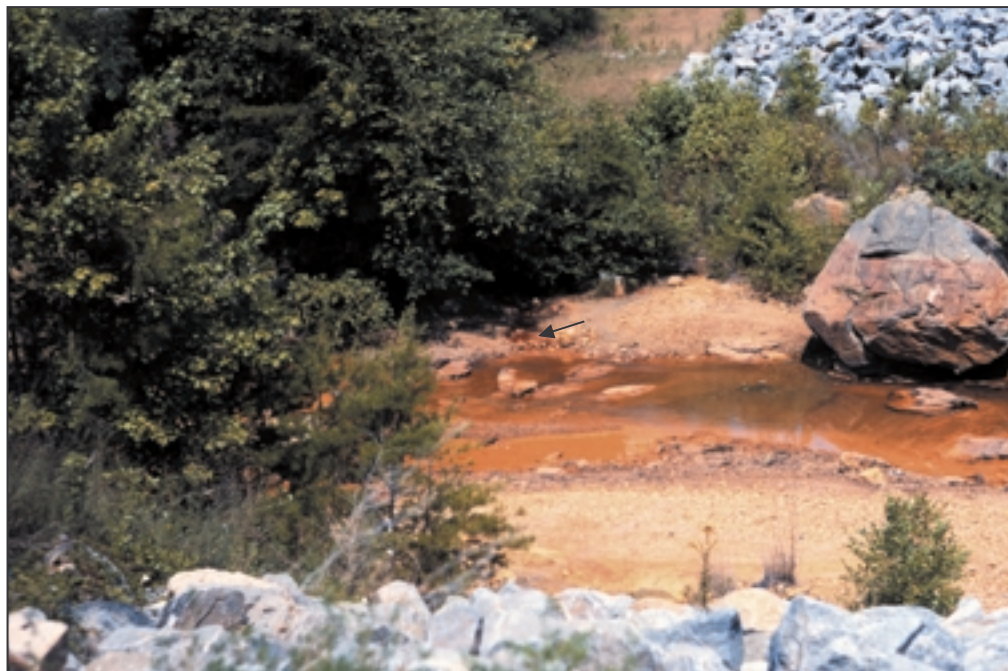
Acid mine drainage site in Virginia. Metal and coal mines within the Chesapeake Bay basin are being studied to learn the limitations of new remote sensing techniques. Contrary Creek in the Piedmont Pyrite Belt in southern Virginia is an ideal test site because it has neutral seeps entering a severely acidified stream. The stream bed is yellow orange from acidic flocculates and precipitates. Dried yellow flocculates extend over the creek banks. In contrast, a neutral tributary in the background (arrow) is red from iron precipitated by bacteria in neutral, iron-rich ground water.
