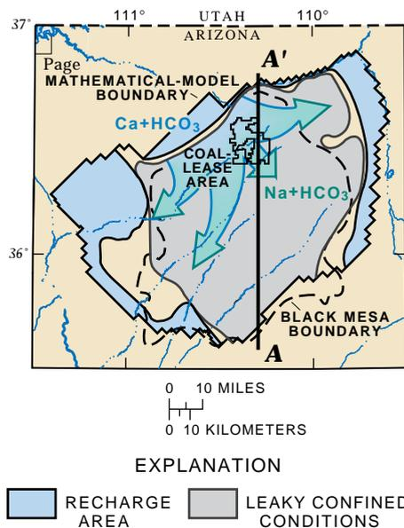
**Figure 2.** Ground-water chemistry—calcium bicarbonate ( $\text{Ca}+\text{HCO}_3$ ) water changes to a sodium bicarbonate ( $\text{Na}+\text{HCO}_3$ ) water.
