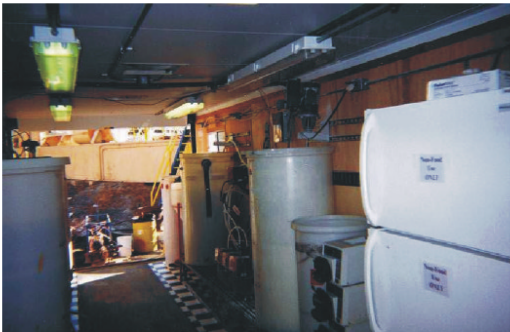
Figure 1-5. Catalyzed cementation process in MWTP demonstration trailer.
