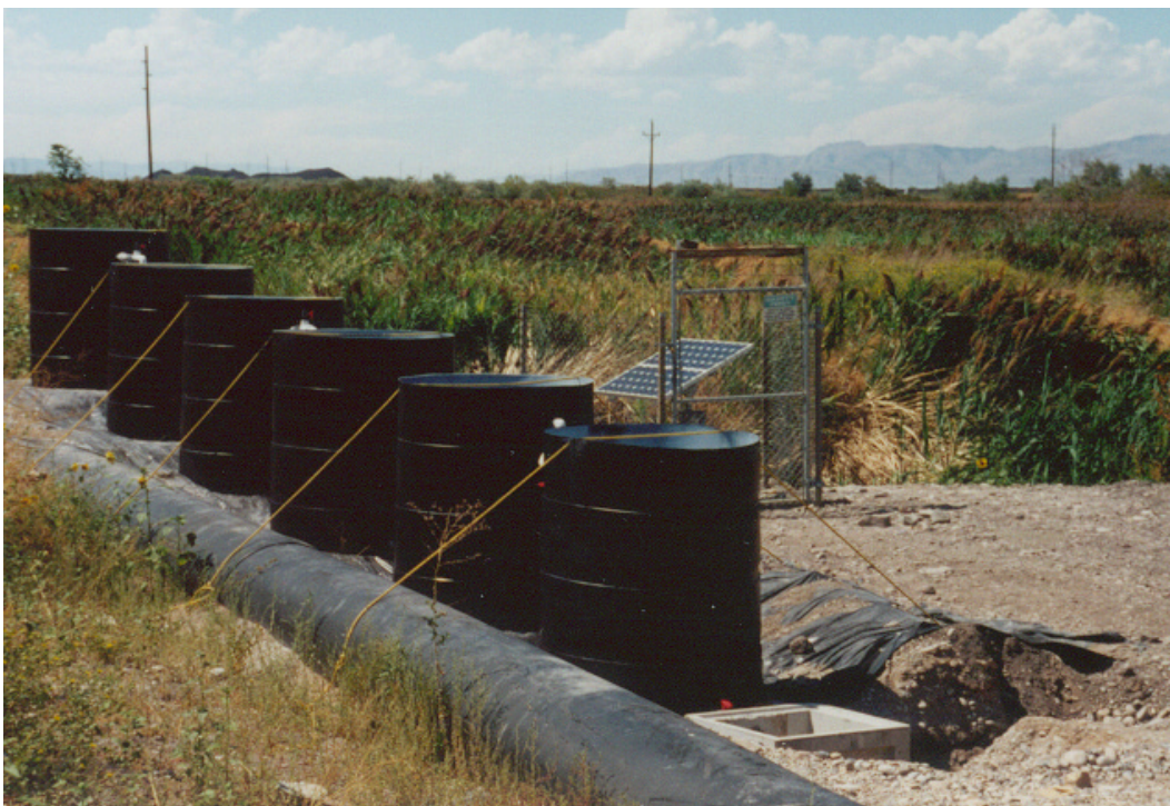
Figure 1-7. Field-scale BSeR™ process reactor.
