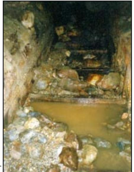
Tunnel sluice with mercury-contaminated sediments.
