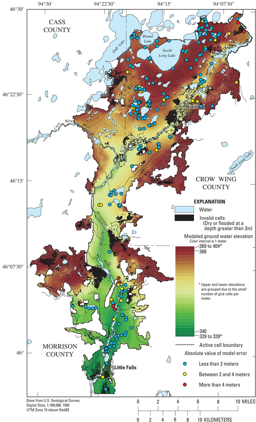
Figure 5. Modeled ground water elevations of the northern model along the Mississippi River between Brainerd and Little Falls in central Minnesota.
