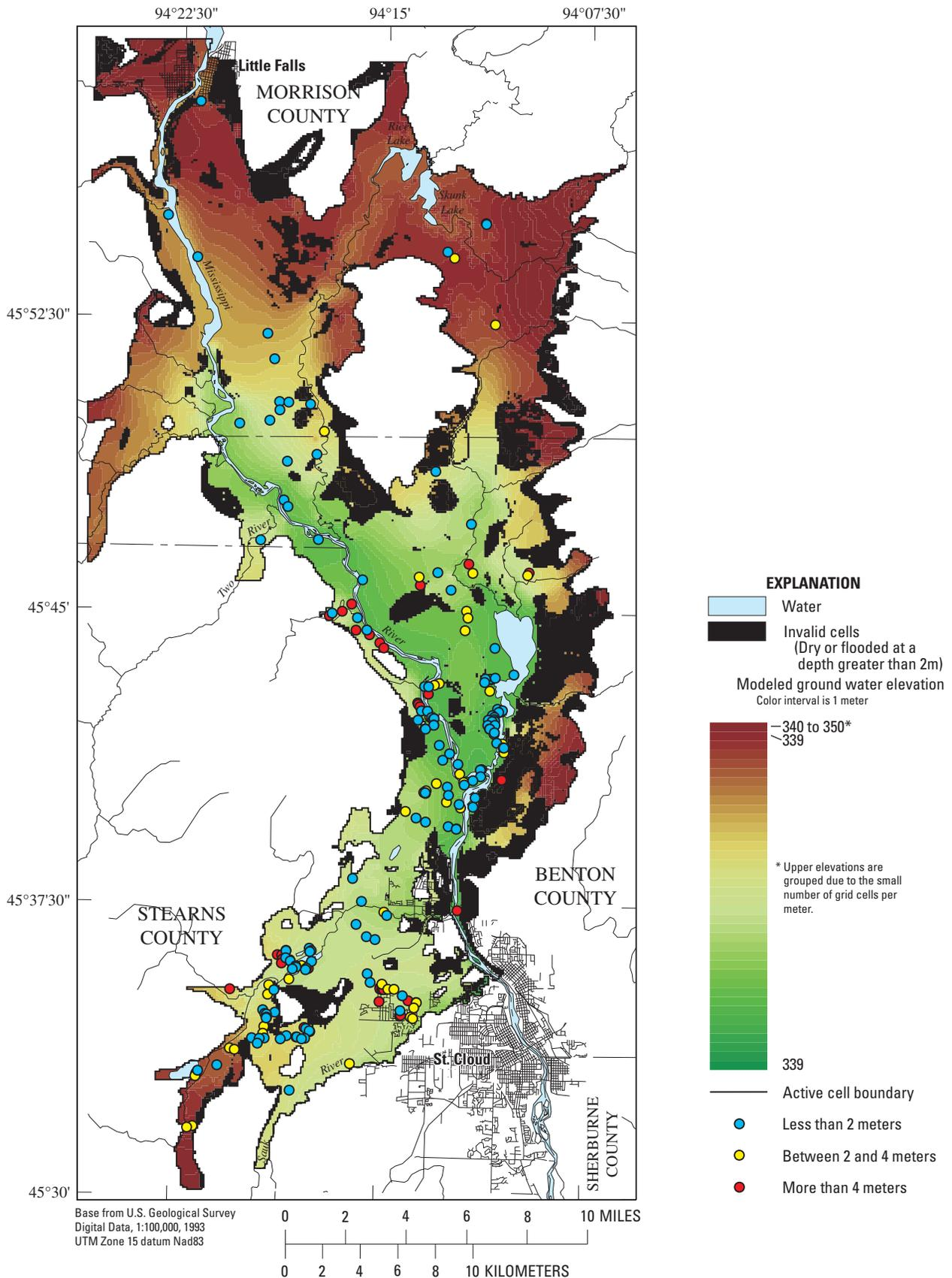
Figure 6. Modeled ground water elevations of the southern model along the Mississippi River between Little Falls and St. Cloud, in central Minnesota
