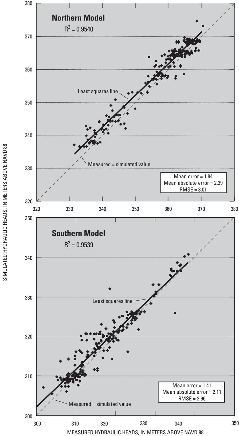
Figure 4. Measured versus simulated water levels in wells for the northern and southern models along the Mississippi River between Brainerd and St. Cloud in central Minnesota [RSME, Root Mean Square Error]
