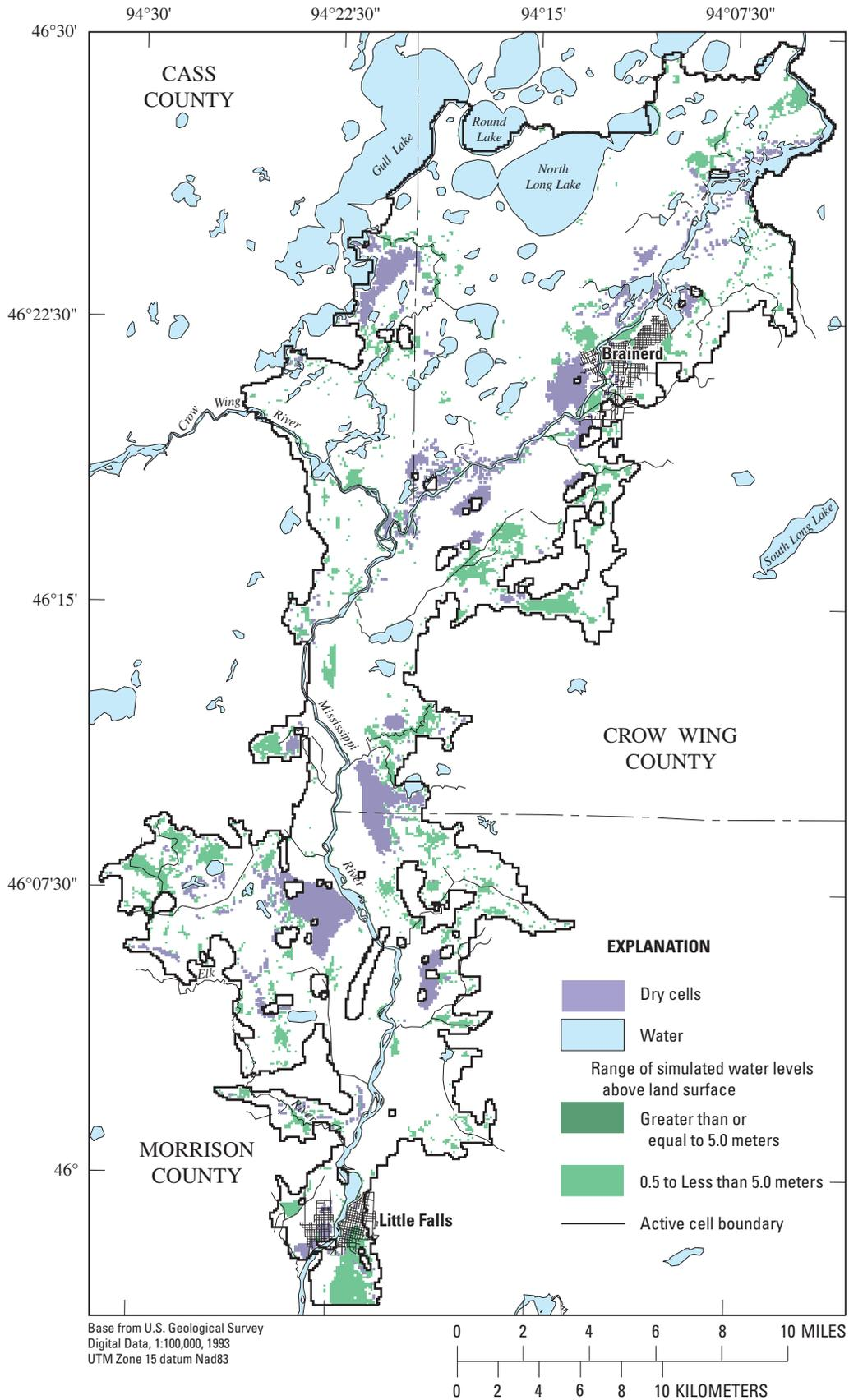
**Figure 7.** Simulated water levels above land surface and dry cells in the northern model along the Mississippi River between Brainerd and Little Falls in central Minnesota
