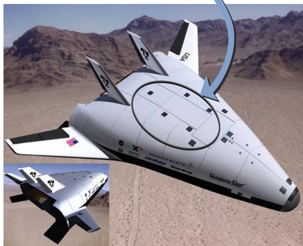
VentureStar reusable launch vehicle, showing where the titanium aluminide metallic thermal protection system will be used.
