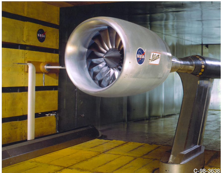
NASA/Allison Engine Company Low Noise Fan test in Lewis' 9- by 15-Foot Low-Speed Wind Tunnel.
