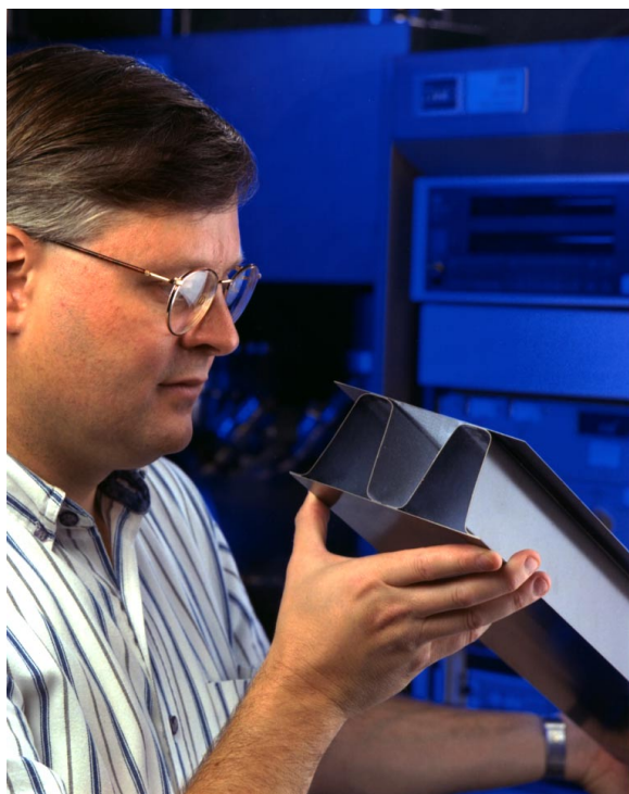
Titanium aluminide truss core subelement manufactured by BFGoodrich Aerostructures group using HSR technologies.
