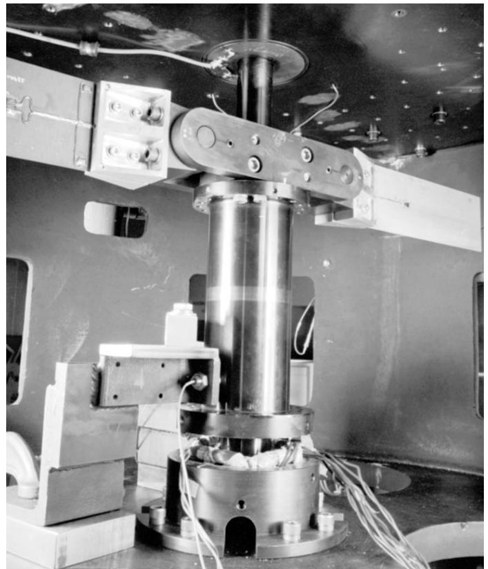
Radial magnetic bearing in NASA Lewis' Dynamic Spin Rig showing viscoelastic damped composite plates attached to the rotor.
