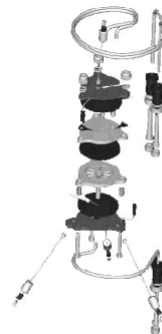
Figure 3. Exploded view of an electrolyzer assembly.
