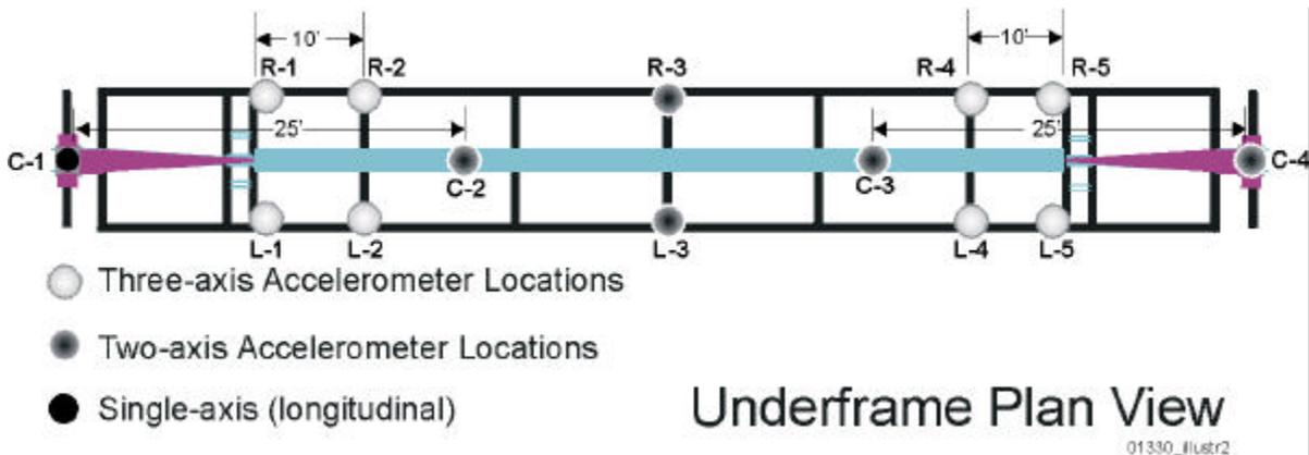
Figure 6.2.1 Schematic Diagram of Accelerometer Locations.
