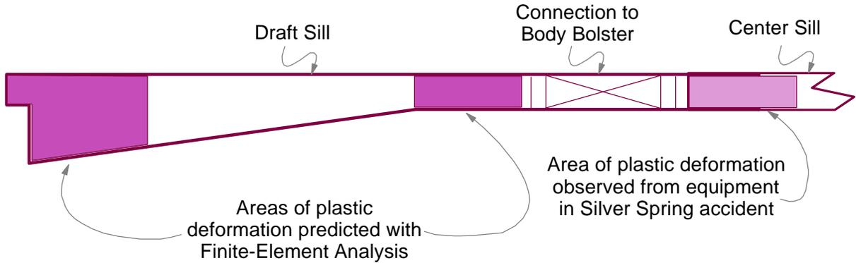
Figure 6.1.1 Potential areas of plastic deformation, draft sill and center sill.
