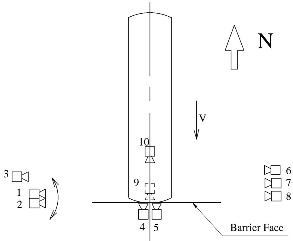
Fig. 6 -3-1 Camera placement
